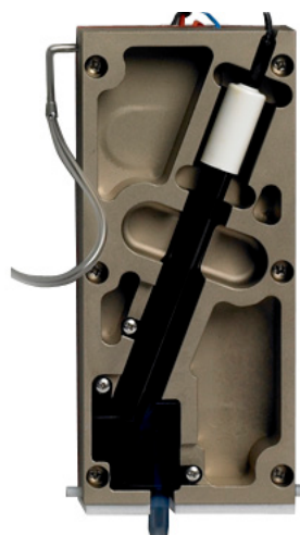
Figure 3 Electrode in temperature-controlled flow cell
