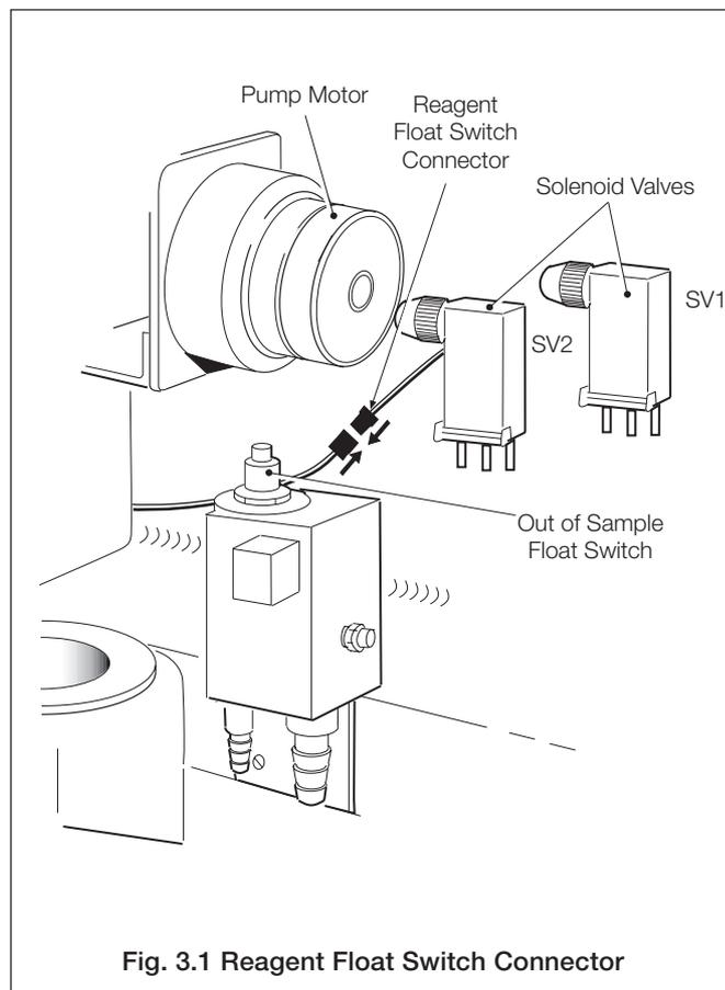
**Fig. 3.1 Reagent Float Switch Connector**
