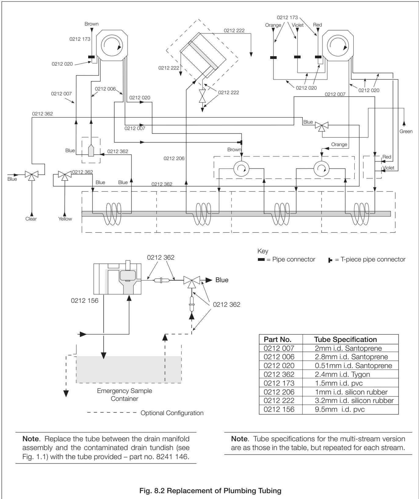
Fig. 8.2 Replacement of Plumbing Tubing
