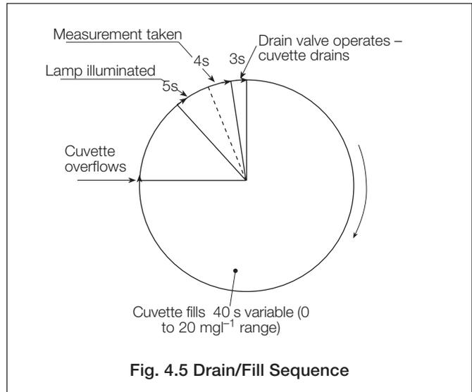
Fig. 4.5 Drain/Fill Sequence
