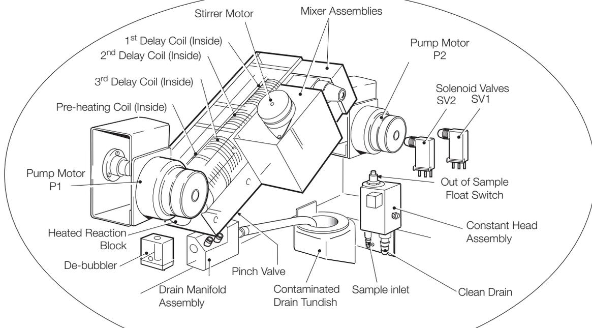
**Internal view of liquid handling section**
