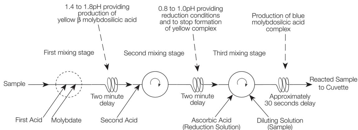
Fig. 4.1 Chemical Schematic
