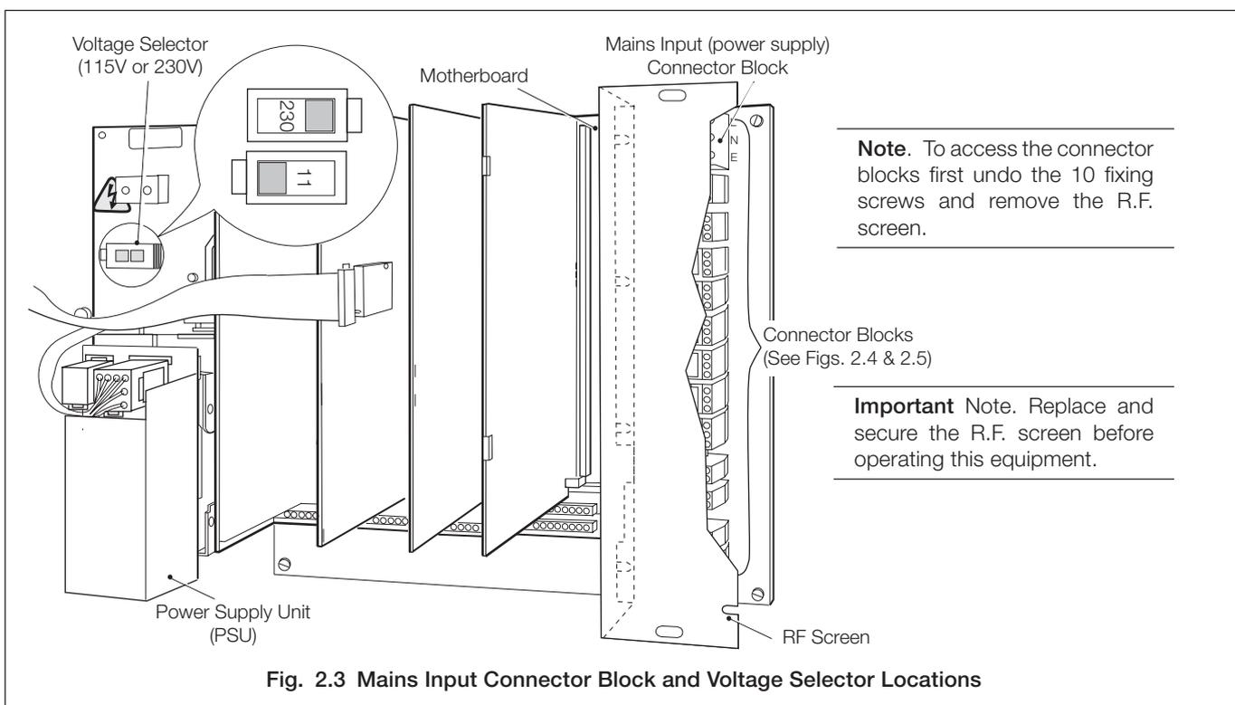
Fig. 2.3 Mains Input Connector Block and Voltage Selector Locations
