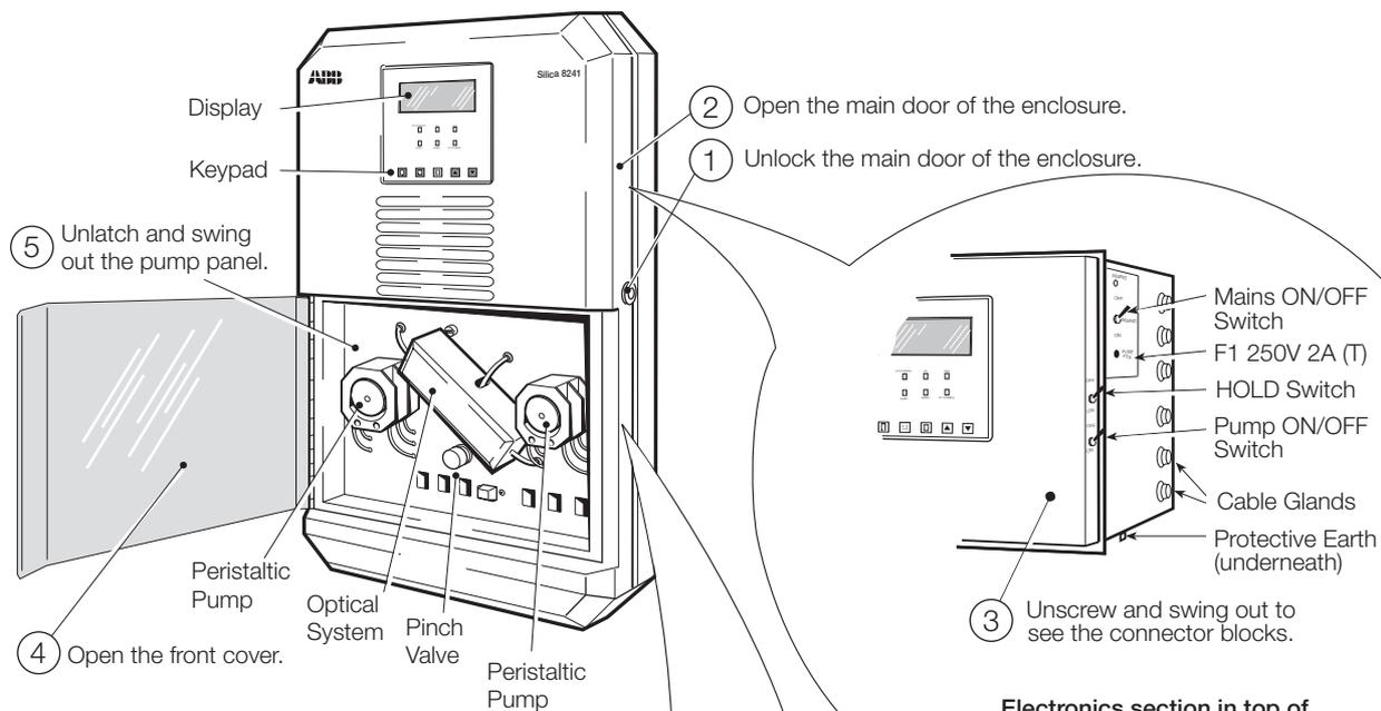
**Electronics section in top of case (see Figs. 2.3 to 2.5 for internal details)**
