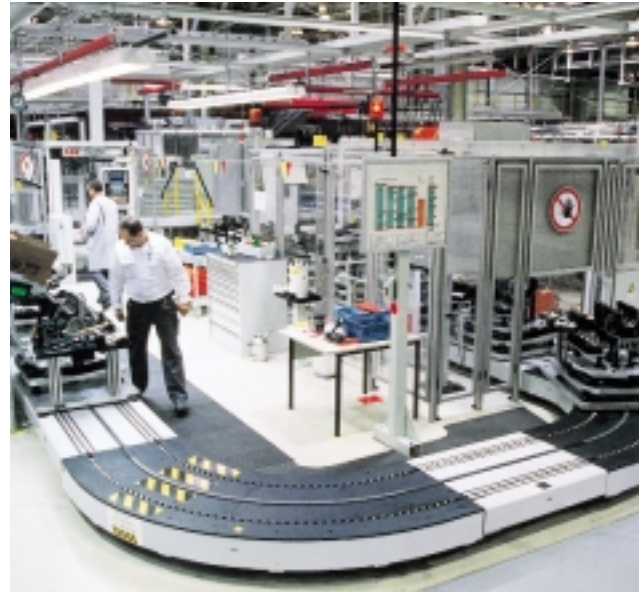
Coupling stations transfer the partly assembled units to the team loops on special pallets. The stations are designed according to ergonomic principles. 5
