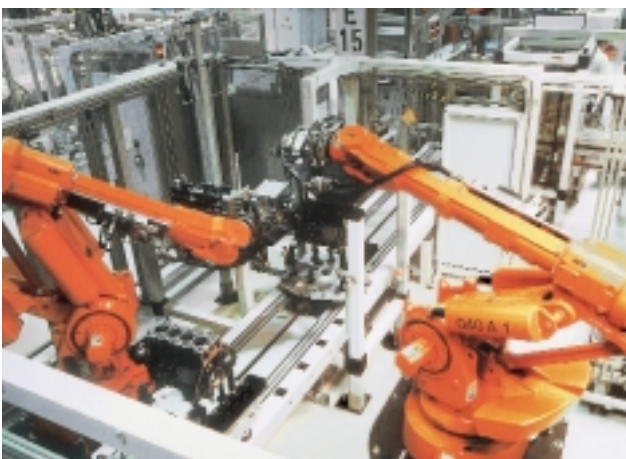
Two jointed-arm robots fitting the injection pumps – an eye-catching feature of the Opel plant in Kaiserslautern 6
