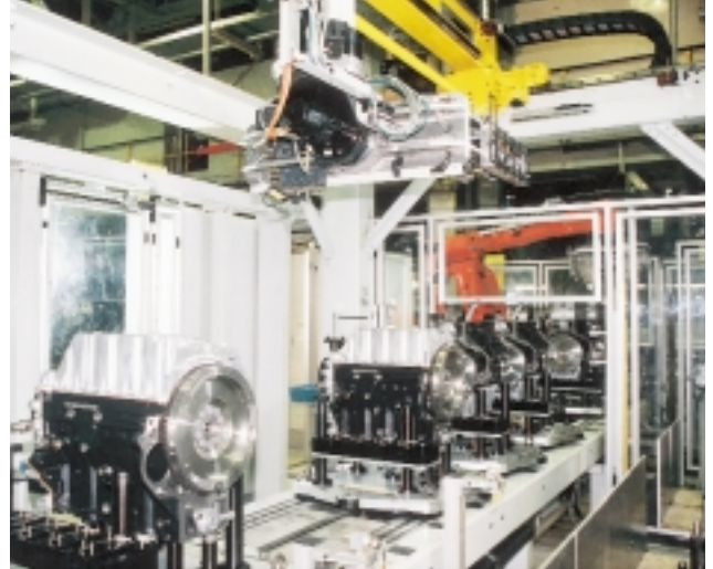
Robots 'marry' the engine blocks and cylinder heads, which arrive from their respective assembly lines.
