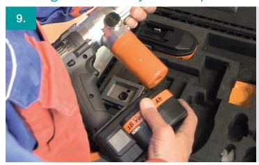
Place the battery in the power unit, as shown in the image.
