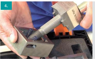
Ensure that the coil springs stay in place.
