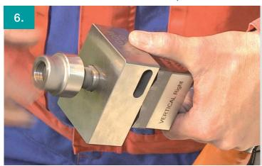
Screw the nut onto the feed rod.
