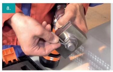
Use the pin to secure the nut in place.
