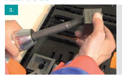
Install the die and punch it onto the feed rod.
