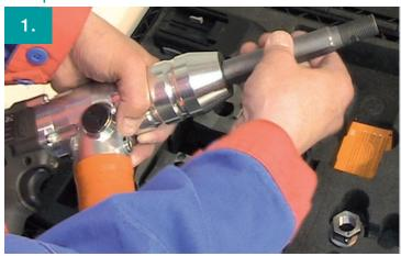
Insert the feed rod into the power unit.
