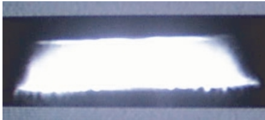
7 Vacuum arc under the influence of a quadrupole axial magnetic field ( I = 31.5 kA; photo taken in the region of the peak current value; contact diameter 68.5 mm; anode at top, cathode at bottom)
