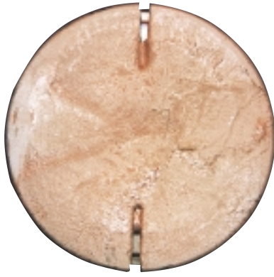
9 Contact surface of a bipolar contact system after multiple short-circuit current interruptions (63 kA; contact diameter 100 mm)
