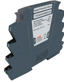
Combined Category D, C, B tested protector (to BS EN 61643) suitable for 3-wire signalling applications which require either a lower in-line resistance, an increased current and/or higher bandwidth. Also suitable for DC power applications less than 0.5 Amps. Available for working voltages of up to 6, 15, 30, 50 and 110 Volts. For use at boundaries up to LPZ 0 to protect against flashover (typically the service entrance location) through to LPZ 3 to protect sensitive electronic equipment.
