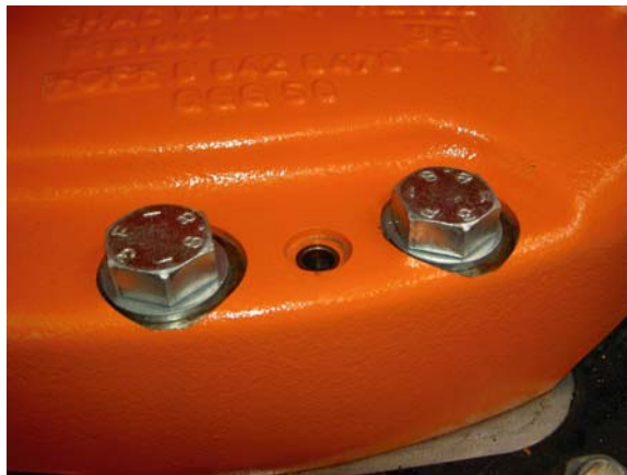
Figure 12 Four Ø12 H8 (depth 12) on radius 400 mm from axis 1 center on robot base.
