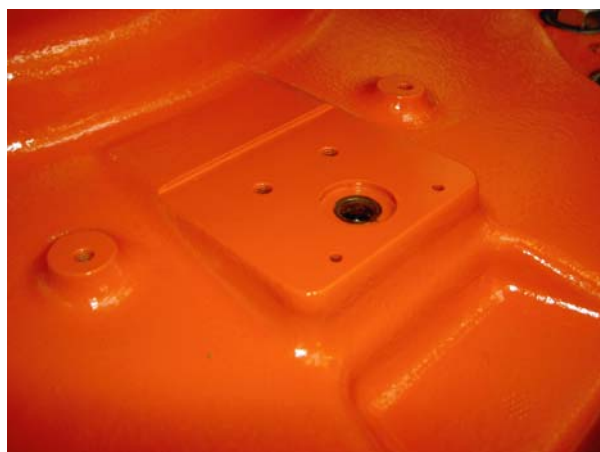
Figure 13 One Ø12 H8 (depth 12) in +x- direction from axis 1 center of robot base.
