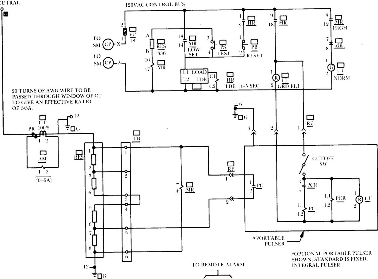
20 TURNS OF AWG WIRE TO BE PASSED THROUGH WINDOW OF CT TO GIVE AN EFFECTIVE RATIO OF 5/5A.
