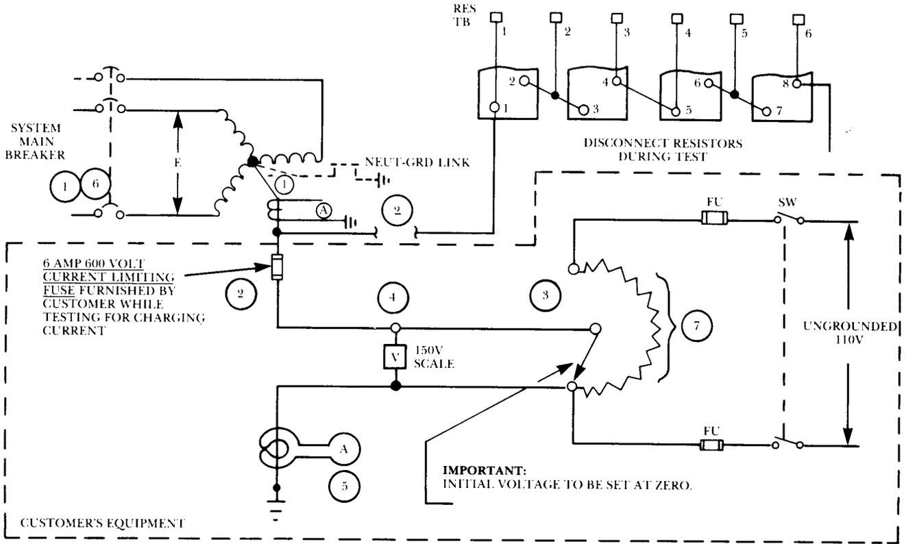
Figure 3. Testing Schematic
