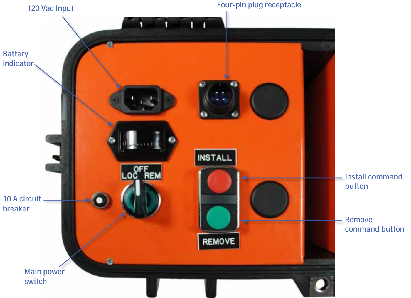
Figure 5-2: RSO Control Panel Components
