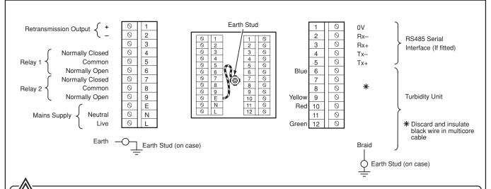
Warning. The power supply earth (ground) must be connected to ensure safety to personnel, reduction of the effects of RFI and correct operation of the power supply interference filter.
