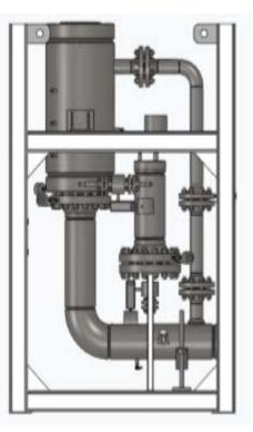
H: 3000mm; W: 1000mm; L: 2000mm Weight: 2700kg
