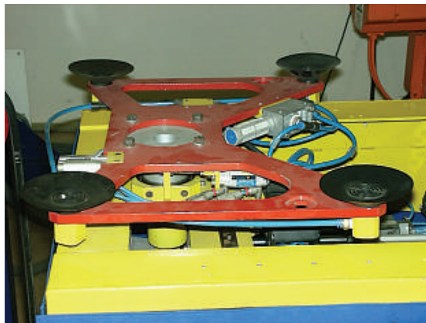
5 The squaring module. Squaring is performed by servo-controlled tools designed to handle fragile products.
