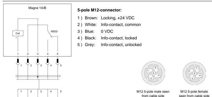
NB: Magne 1A/B can be connected in series using M12-3A.
