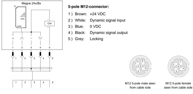
NB: Magne 2Ax/Bx can be connected to the AS-i bus using Urax B1R.
