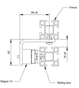
Installation tolerance (sliding door)
