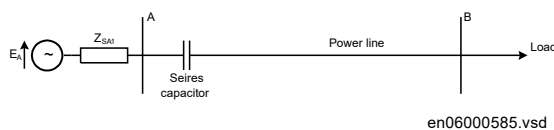
Figure 76: A simple radial power system
