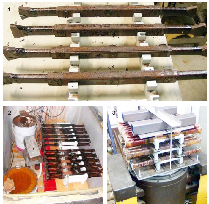
Figure 10. 1 Aged test bars (steel covers rusted due to moisture handling) | 2 Test bars in moisture chamber | 3 Test bars on vibration bench
