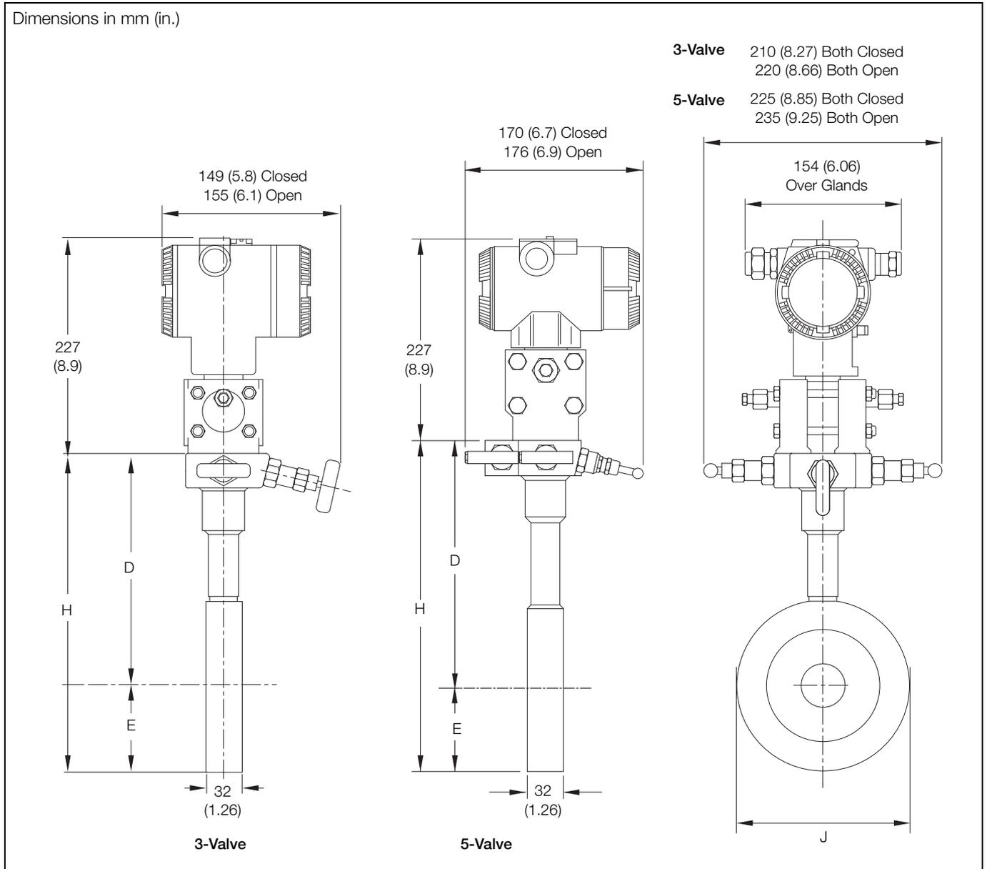
Fig. 2.2 OriMaster V (Design Level 2) 3-Valve and 5-Valve Dimensions
