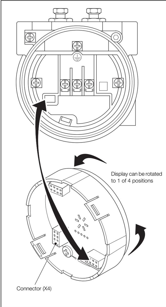
Fig. 2.8 Integral Display Positioning
