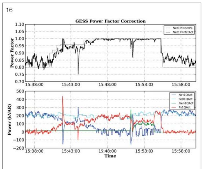
16 GESS Power Factor Correction. Upstream network power factor (Net1PwrFctAct), power factor setpoint (Net1PfnomPa) and reactive power (Net1QAct), downstream feeder reactive power (Fed1QAct), generator reactive power (Gen1QAct) and PowerStore reactive power (Ps1QAct) during power factor correction.
