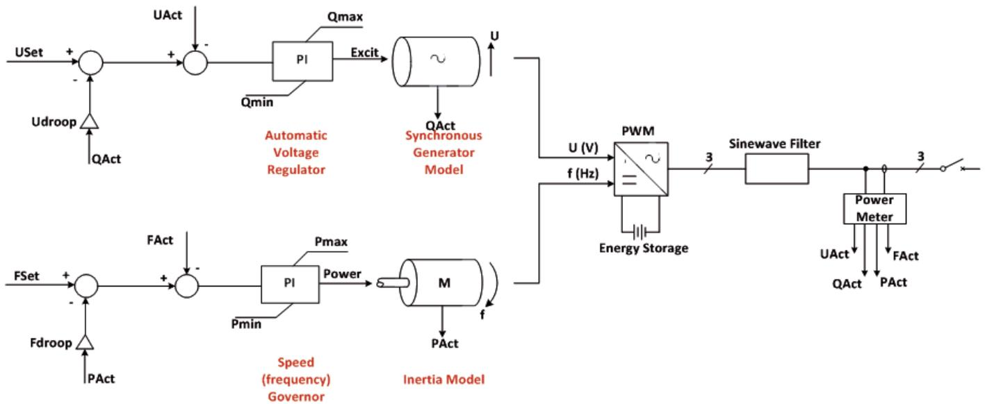
9 Software AVR and Governor models used in the PowerStore Virtual Generator Mode
