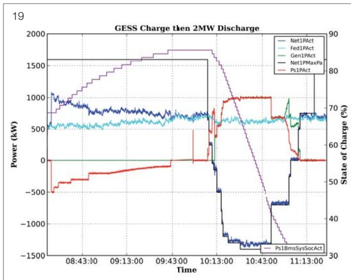
19 GESS charging then 2MW discharge. Upstream feeder power (Net1PAct) and maximum power setpoint (Net1PMaxPa), downstream feeder power (Fed1PAct), Generator power (Gen1PAct), PowerStore power (Ps1PAct) and battery system state-of-charge (Ps1BmsSysSocAct) during charge then full power 2MW discharge
