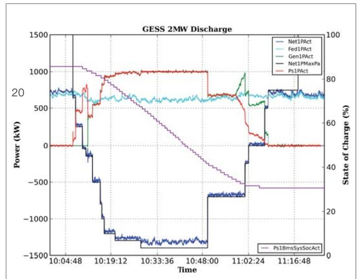
20 GESS 2MW discharge. Upstream feeder power (Net1PAct) and maximum power setpoint (Net1PMaxPa), downstream feeder power (Fed1PAct), Generator power (Gen1PAct), PowerStore power (Ps1PAct) and battery system state-of-charge (Ps1BmsSysSocAct) during full power 2 MW discharge.
