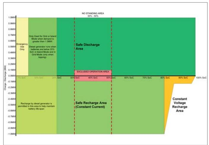
**10 GESS battery management scheme detailing charging and discharging regions. During operation the GESS does not maintain the state of charge of the batteries within the 'no standing area', instead charging or discharging through the region as required.**
