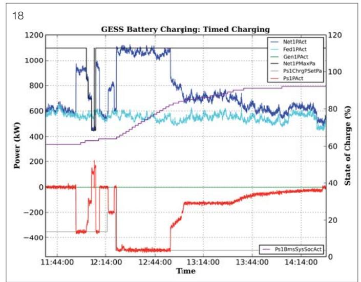
18 GESS Battery Charging: Timed Charging. Upstream feeder power (Net1PAct) and maximum power setpoint (Net1PMaxPa), downstream feeder power (Fed1PAct), generator power (Gen1PAct), PowerStore power (Ps1PAct) and PowerStore maximum charging power (Ps1ChrgPSetPa) and battery system state-of-charge (Ps1BmsSysSocAct) during timed charging
