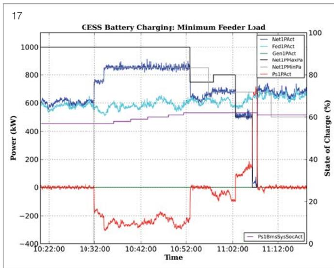
17 GESS Battery Charging: Minimum Feeder Load. Upstream feeder power (Net1PAct), maximum power setpoint (Net1PMaxPa) and minimum power setpoint (Net1PMinPa), downstream feeder power (Fed1PAct), generator power (Gen1PAct), PowerStore power (Ps1PAct) and battery system state-of-charge (Ps1BmsSysSocAct) during charging while maintaining minimum feeder load
