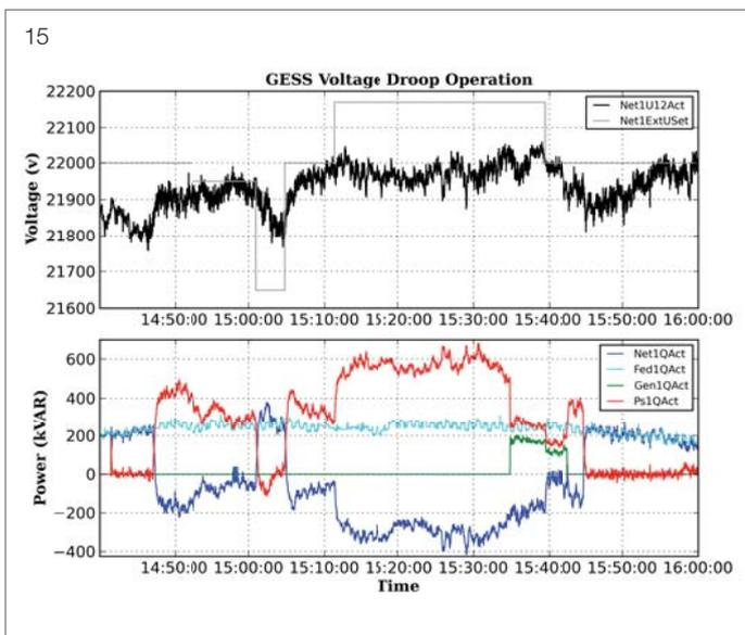
15 GESS Voltage Droop Operation. Upstream feeder voltage (Net1U12Act), voltage droop setpoint (Net1ExtUSet) and reactive power (Net1QAct), downstream feeder reactive power (Fed1QAct), generator reactive power (Gen1QAct) and PowerStore reactive power (Ps1QAct) during voltage droop operation
