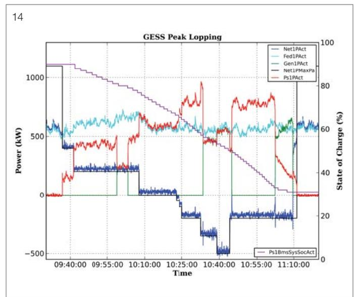
14 GESS Peak Lopping. Upstream feeder power (Net1PAct) and maximum power setpoint (Net1PMaxPa), downstream feeder power (Fed1PAct), Generator power (Gen1PAct), PowerStore power (Ps1PAct) and battery system state-of-charge (Ps1BmsSysSocAct) during peak lopping.
