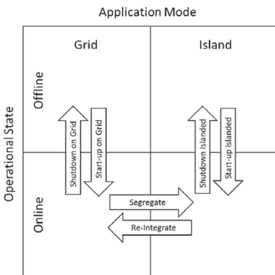
limits. During the synchronization and closure of the upstream breaker, the GESS continues to supply the downstream load resulting in a ‘bumpless’ transition. The GESS then can continue to providing grid supply and support, begin charging the battery bank or ramping down the output of the system to full transfer of the supply back to the grid.
