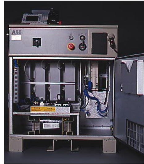
The electronic design results in a clear and uncluttered layout for high reliability and easy access.
