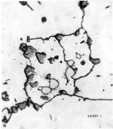
a. As received. b. After 48 h, 650° C., 20 kg/mm 2 . Figs. 3a and 3b. — Translation movements in the cleavage surfaces and grain boundaries of a high-alloy steel as a result of continuous heat and stress. (Magnified 1100 ×) These translation movements caused this high-alloy Cr Ni steel to become completely brittle.
