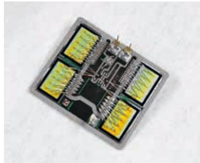
The new concept is dubbed BIGT (bimode insulated-gate transistor). The main target application is hard-switching mainstream inverters. First prototype devices with voltage ratings above 3,300 V have demonstrated high power densities and an improved overall performance.
