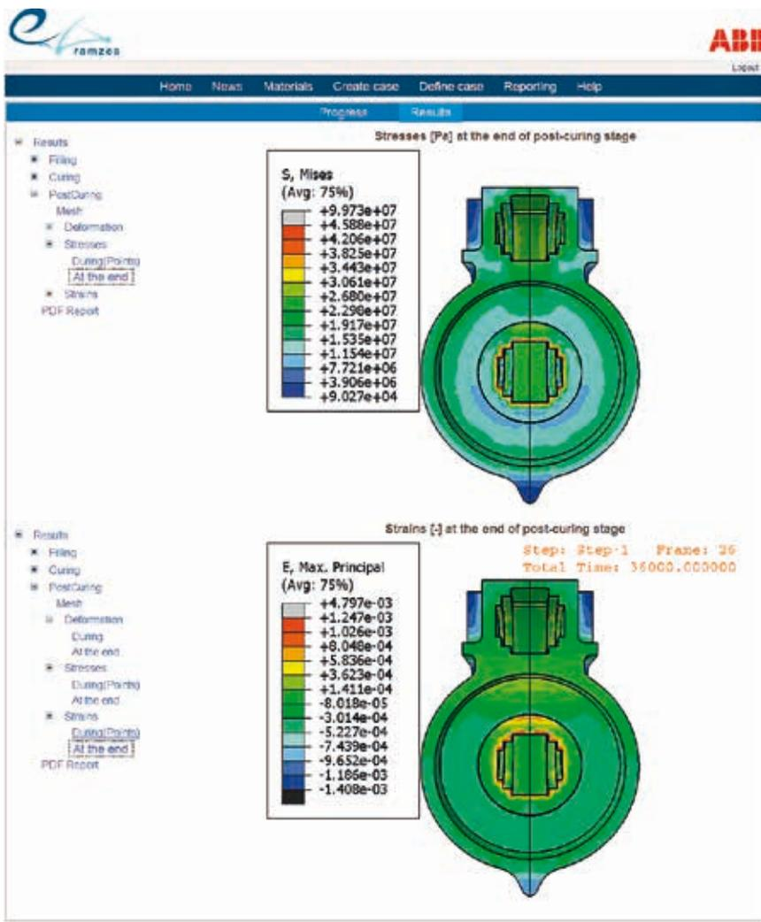
ing products manufactured by reactive molding. The tool allows ABB engineers to observe the influence on the product and its manufacture caused by changes in the design of product and mold as well as by modifications of the process parameters. Furthermore it achieves this without requiring interference in the real production process.
