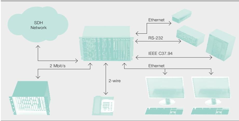
**FOX615 multiservice node:** Different user interfaces can be directly connected to the SDH communication backbone.
