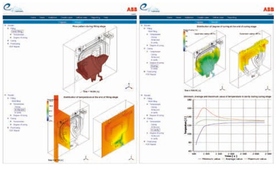
It is worth noting that reactive molding simulations are known to be numerically unstable – even when performed manually – due to the complexity of phenomena involved in the process. In the meantime, eRAMZES monitors and automatically controls the solution convergence ensuring an excellent stability of computations without requiring additional user actions. In this way one of the biggest challenges during the tool’s development became one of its most significant achievements.
