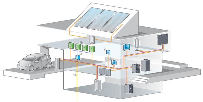
meter. Utility information, in the form of a 24 hour forecast of the electricity price and CO<sub>2</sub> emissions, is sent to the ESI daily. Using household preferences together with meter and utility information, the ESI's energy management system's logic schedules the household's electric loads with the goal of minimizing electrical consumption costs and environmental impacts while still retaining comfort.
