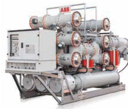
This new GIS features a fast, single-interrupter dual motion circuit breaker and is designed for current ratings of up to 5,000 amperes (A). It provides protection for power networks with rated short-circuit currents of up to 63 kilo amperes (kA).
