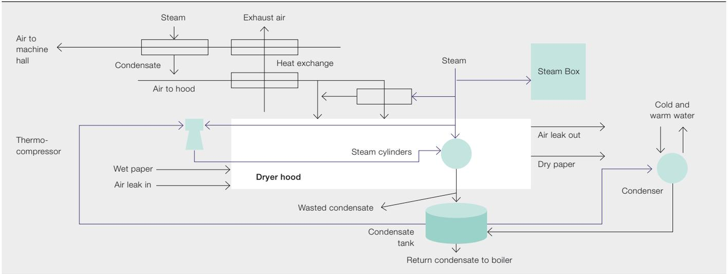
The main steam usage is, as expected, in the different steam groups, but, in this paper machine, more than 10 percent of the total steam energy goes to the condenser. An industry-typical value would be under 3 percent, so energy efficiency improvements here are obviously feasible.
