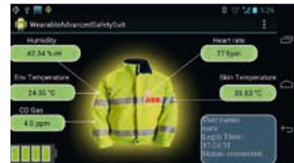
conditions such as gas levels or temperature as well as the health of the wearer. Via augmented reality applications on mobile phones, tablets or special glasses, the field technician can get background information to make his work more efficient and safer.
