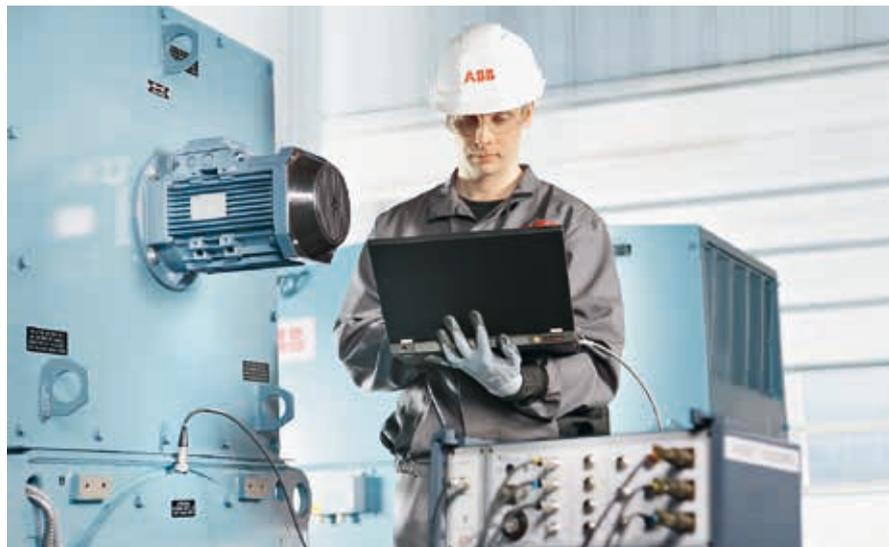
vibration, voltage, current and temperature sensors. Analysis software consists of libraries of algorithms that are used collectively to achieve the best possible discrimination of defects.
