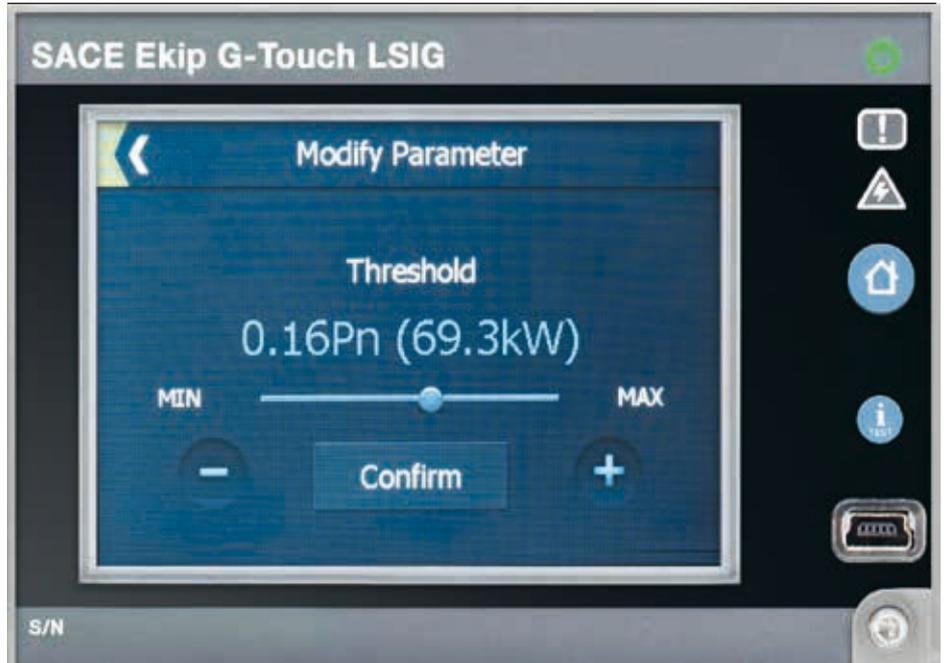
ceeding the power limit. The power controller constantly optimizes the number of disconnected loads, while continuously trying to supply the largest possible load to the plant. Controllable loads are connected and disconnected by slave breakers, either of Emax 2 or legacy type, which are opened and closed
