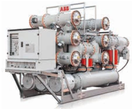
This new GIS features a fast, single-interrupter dual motion circuit breaker and is designed for current ratings of up to 5,000 amperes (A). It provides protection for power networks with rated short-circuit currents of up to 63 kilo amperes (kA).
