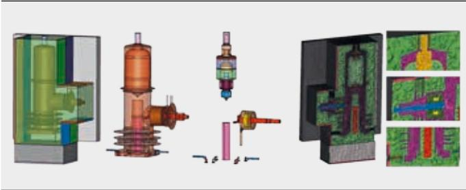
8 Geometry of current transformer (left) and its discretization in ABAQUS (right)
