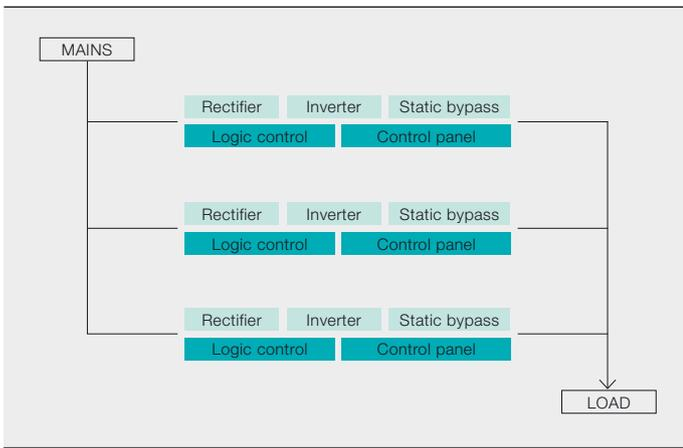
which makes the parallel system fully and truly redundant. With all of the critical components duplicated and distributed between individual units, potential single points of failure are eliminated. System uptime is further maximized by the true safe-swap modularity of the modules.
