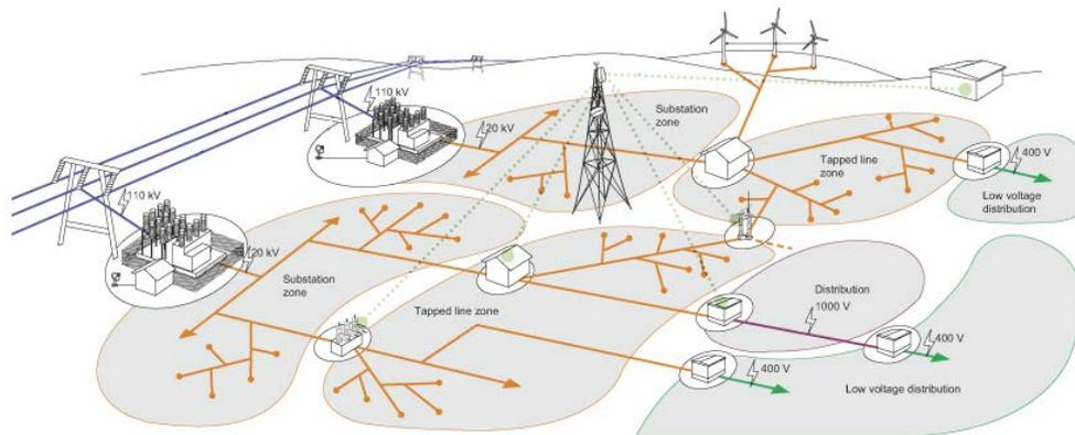
Figure 1. Main principle of the Zone Concept
