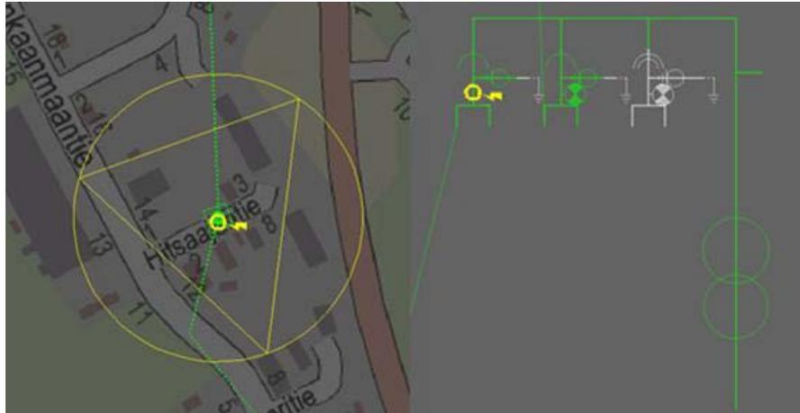
Figure 2. Remotely controlled CSS with fault indication in DMS system
