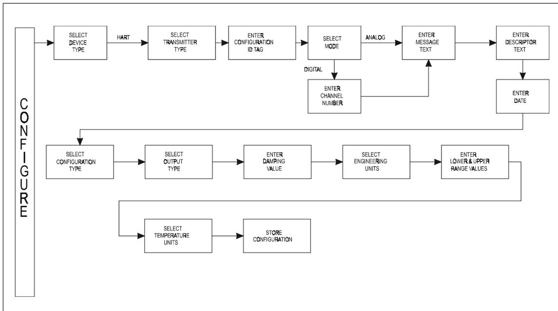
Figure 1. Configuration Flowchart (600T & 600T EN)
