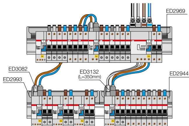
Busbars supplied by means of cable terminal under the head of the circuit-breaker's terminal and branching with parallel module
