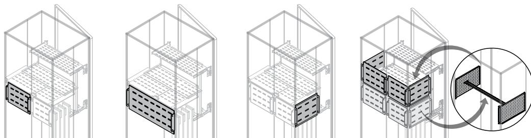
As an alternative to the PLVS... vertical side segregations, in the case of main circuit-breakers (Tmax T5, T6, T7), use the PMCS... side connection module for fixing terminal extensions and the relative fixing bshelves PBMC0002 (page 4/40).
