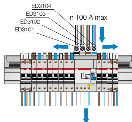
Busbars supplied from above by means of terminals installed laterally
