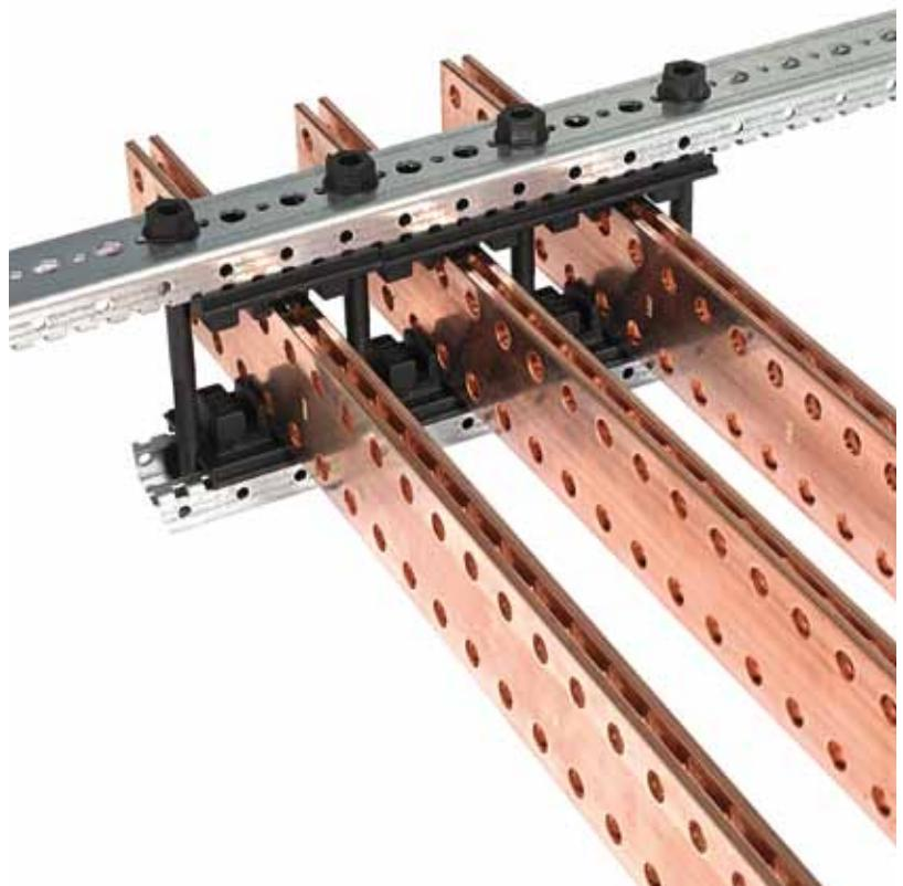
The center distance between phases can be increased by 12.5mm by simply sliding the insulation supports along the crosspieces. When the distance between phases is increased, the length of the closing crosspiece must also be increased.
