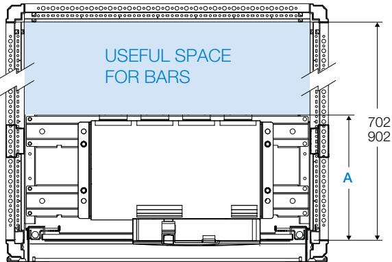
To find the useful space available for the installation of the busbars, according to depth of the structure, subtract the depth of the breaker (A or B) depending on the version shown in the following table.
