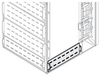
**NEW Lateral segregation in structure with intermediate upright**
