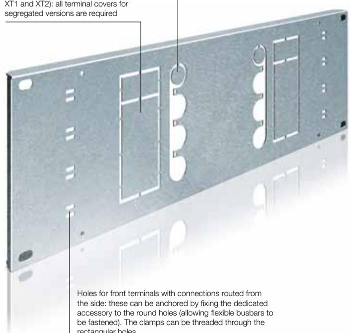
Holes for front terminals with connections routed from the side: these can be anchored by fixing the dedicated accessory to the round holes (allowing flexible busbars to be fastened). The clamps can be threaded through the rectangular holes.
