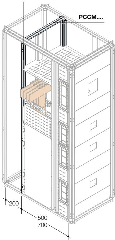
Structure with rear cable compartment: to be realized by means of 2 crosspieces for structure PCCM.... and 2 uprights for internal cable compartment PUCM.... o PUCS....
