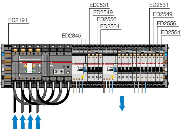
Power supply by means of circuit-breaker supplied from below
