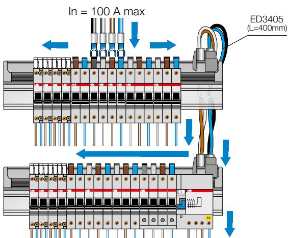
Busbars supplied by means of terminals installed centrally
