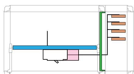
Horizontal circuit-breaker with front/rear terminals
