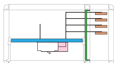
Horizontal circuit-breaker with front/rear terminals
