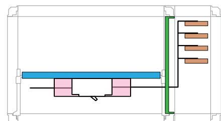
Horizontal circuit-breaker with front terminals side outputs
