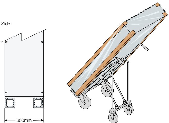
Check the center of gravity before handling structures measuring L=800/1000mm (with internal or external cable compartment) containing busbar systems.
