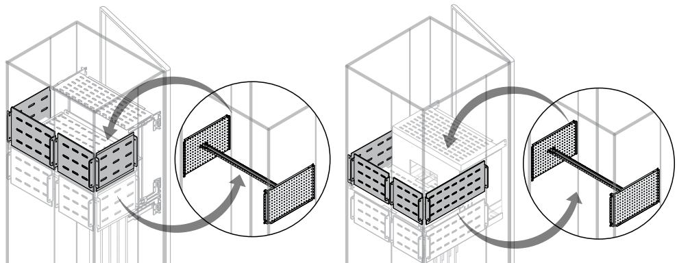
As an alternative to the PLVS... vertical side segregations, in the case of main circuit-breakers, use the PMCS... side connection module for fixing terminal extensions and the relative fixing bshelves PBMC0002 (page 4/40).
