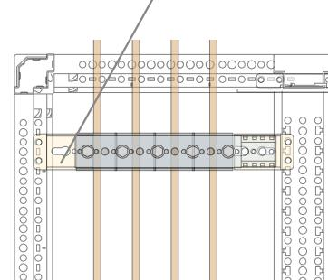
\* The new bracket, PBBU0008 is not compatible with the old ones (PBBT0008, PBBV0008, PBBH0004), on the same busbar system, both horizontal and vertical, it is not possible the coexisting between old and new ones. The fixing of the crosspieces for busbar system must be done with only one kind of bracket.
