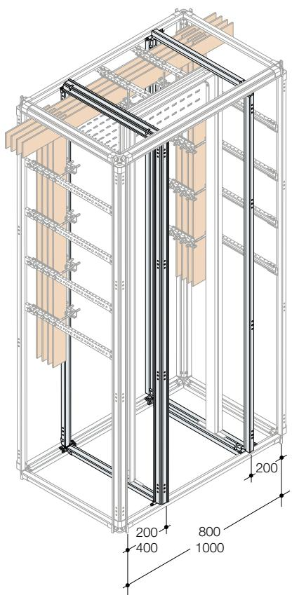
Structure with double internal cable compartment: to be realized by means of crosspieces for internal cable compartment PCCS.... and uprights for internal cable compartment PUCM.... o PUCS....
