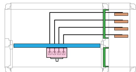
Vertical circuit-breaker with front terminals
