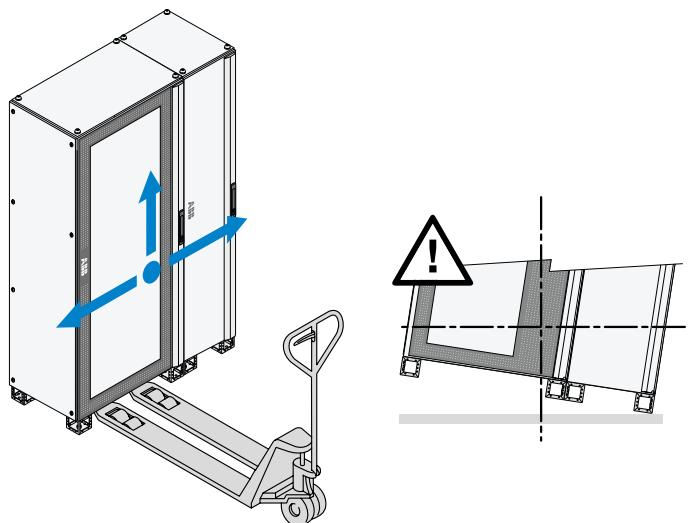
For extra safety, it is advisable to fasten the switchboard to the lift truck when using this type of vehicle for transport.
