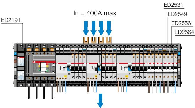
Busbars supplied from above by means of a 4P feeder module installed centrally
