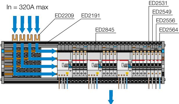
Power supply by means of circuit-breaker supplied from above
