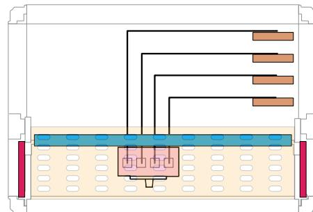
Vertical circuit-breaker with front terminals
