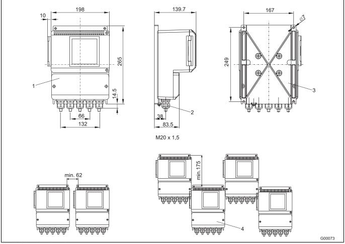
Fig. 78 (Dimensions in mm)
