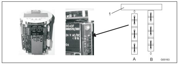
Fig. 53 Setting the pulse output using jumpers
