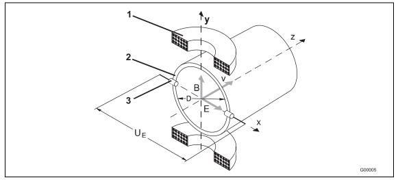
Fig. 5: Electromagnetic flowmeter schematic
