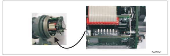
Fig. 54 Position of DIP switches using example of FXE4000 (COPA-XE)
