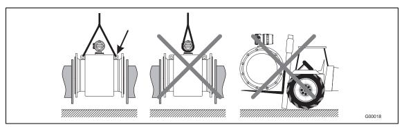
Fig. 9: Transport of flanged units larger than DN 400
