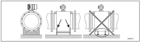
Fig. 21: Support for meter sizes larger than DN 400
