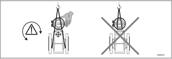
Fig. 8: Transport of flanged units smaller than DN 450
