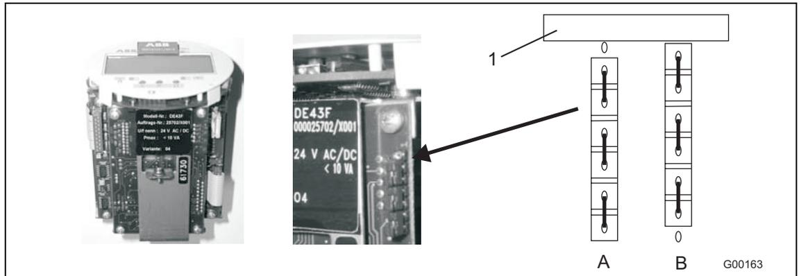
Fig. 53 Setting the pulse output using jumpers
