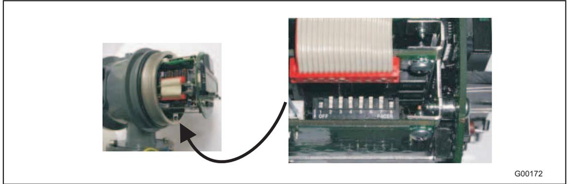
Fig. 54 Position of DIP switches using example of FXE4000 (COPA-XE)
