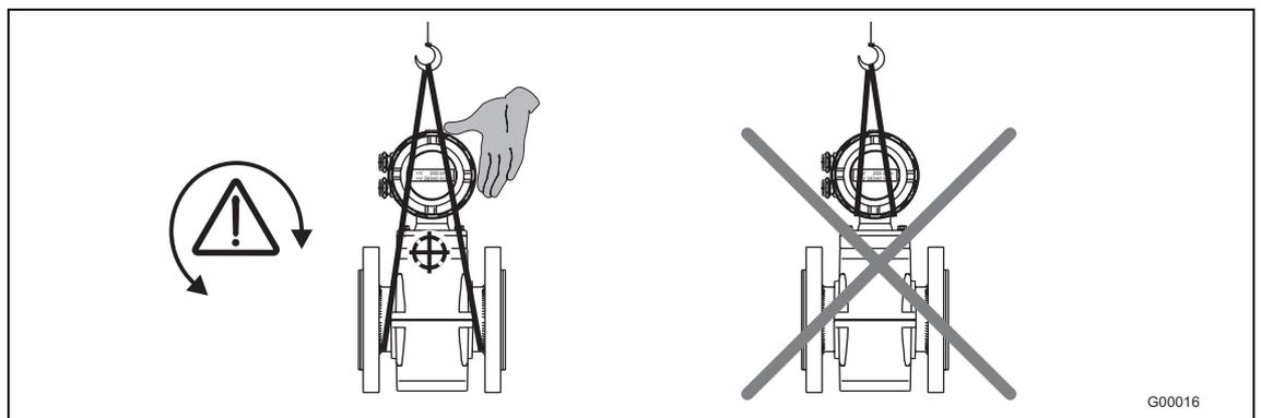
Fig. 8: Transport of flanged units smaller than DN 450
