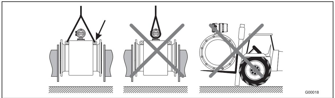
Fig. 9: Transport of flanged units larger than DN 400
