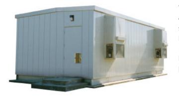
The PDC-6000 is a prefabricated modular, skid-mounted enclosure for switchgear and auxiliary equipment. As a self-contained unit, it is completely coordinated, assembled and tested in controlled factory environment. With integral transformers, close-coupled to switchgear or with bus duct connections, a PDC-6000 can serve as a complete unit substation
