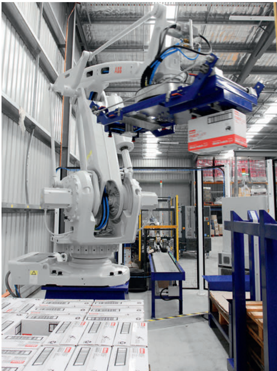
Decor uses the IRB 660 four-axis palletizing robot to palletize all of the product.
