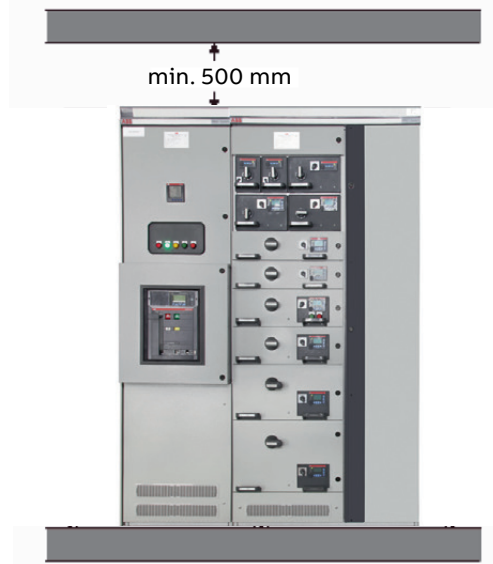
32 Free space above cubicle
