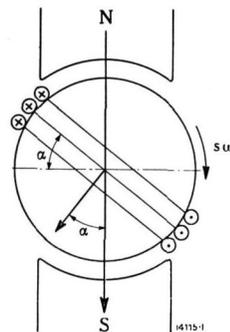
Fig. 1.—Simplified diagram of a synchronous motor.
