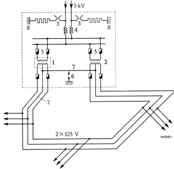
Fig. 14. — Substation with transformers.
