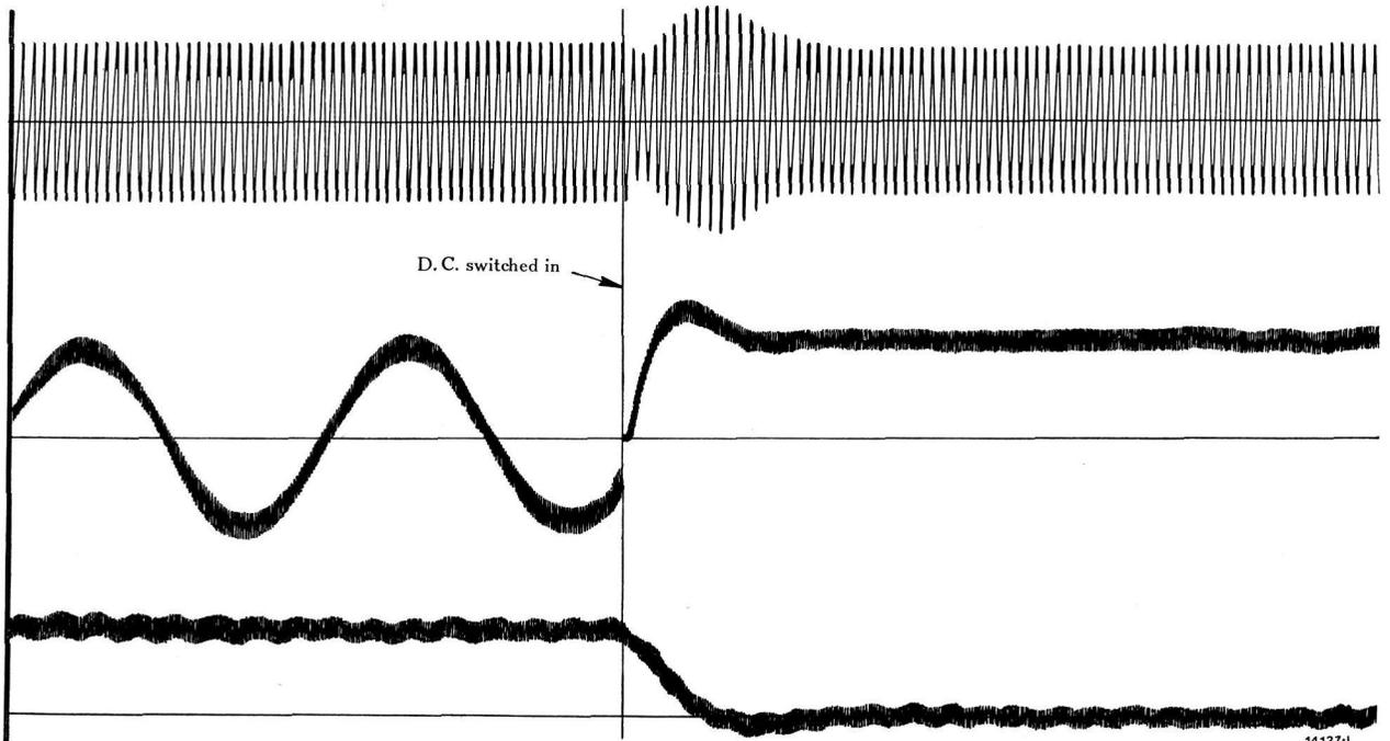
Fig. 12a. — Oscillogram showing the stator and rotor currents and the slip during synchronisation of a 100-kW motor-generator set. Switching in takes place in the most favourable position.
