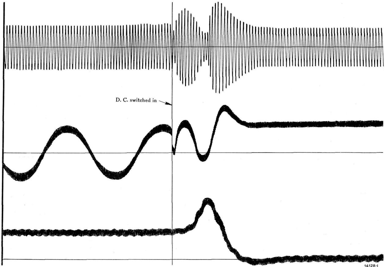
Fig. 12b. — Oscillogram showing the stator and rotor currents and the slip during synchronisation of a 100-kW motor-generator set. Switching in takes place in the most unfavourable position.
