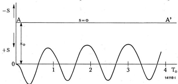
Fig. 2. — Periodic variations of slip if direct current is switched on when  $\alpha = 180^\circ$ .
