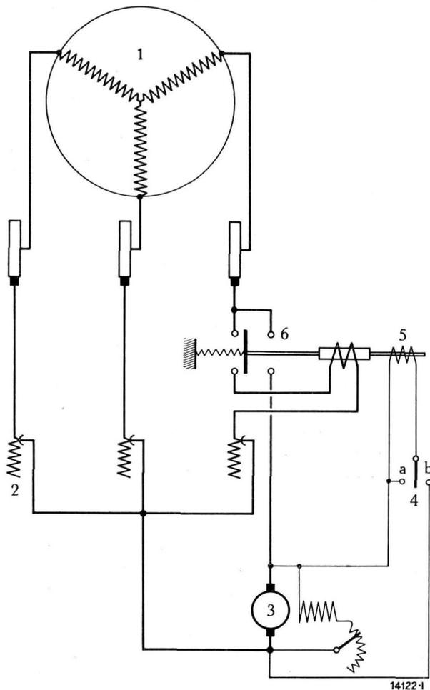
Fig. 8. — Brown Boveri automatic synchronising device.
