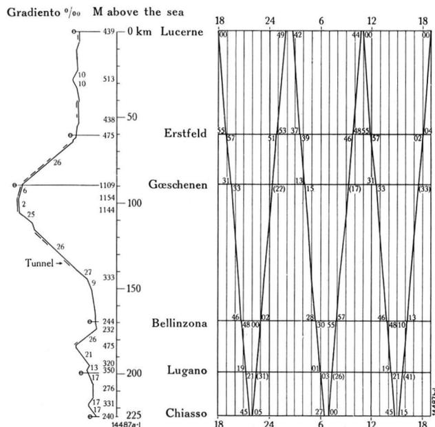
Fig. 1. — Time-table of the official trials of the 1B-B1 locomotive on September 23 and 24, 1922.
