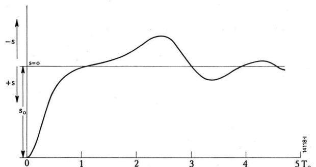
Fig. 4. — Periodic variations of slip if direct current is switched in when  $\alpha = 0$ , the excitation being the same as in Fig. 2.
