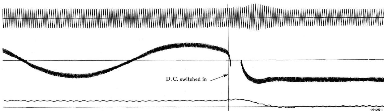
Fig. 11a. — Oscillogram showing the stator and rotor currents and the slip during synchronization of a 1000-kW motor-generator set. Switching in takes place in the most favourable position.
