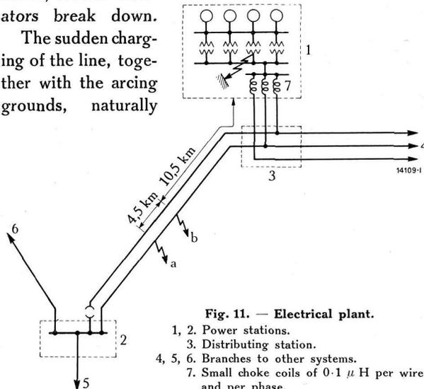
Fig. 11. — Electrical plant.
