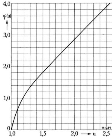
Fig. 9. — Auxiliary curve for calculating the minimum excitation permissible.
