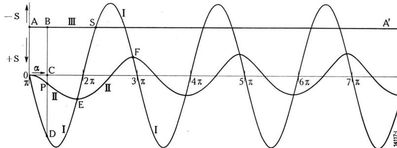
Fig. 3. — Accelerating and retarding torques when several pole spaces are slipped, the conditions being the same as in Fig. 2.
