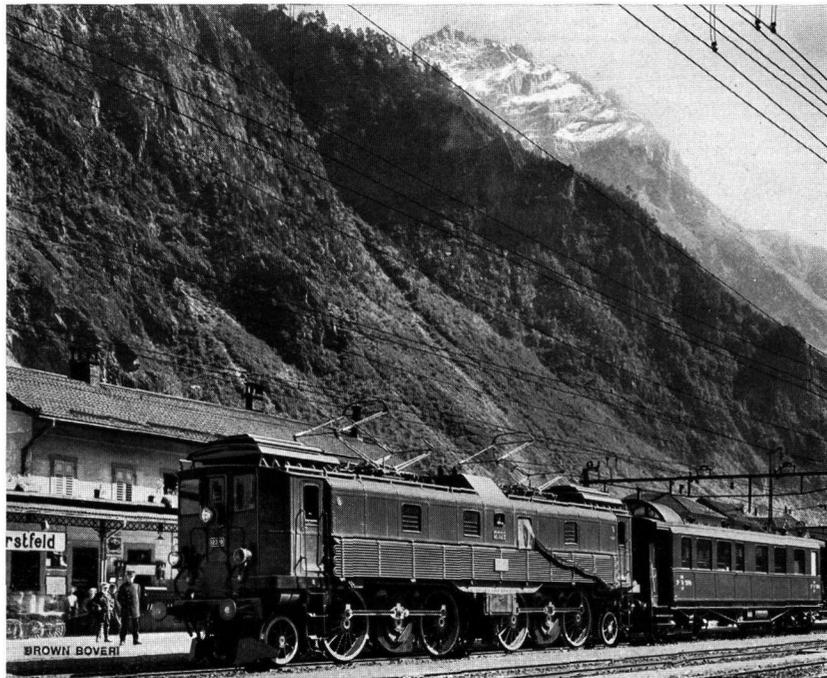
Fig. 2. — 1B-B1 locomotive during trials with dynamometer car.
