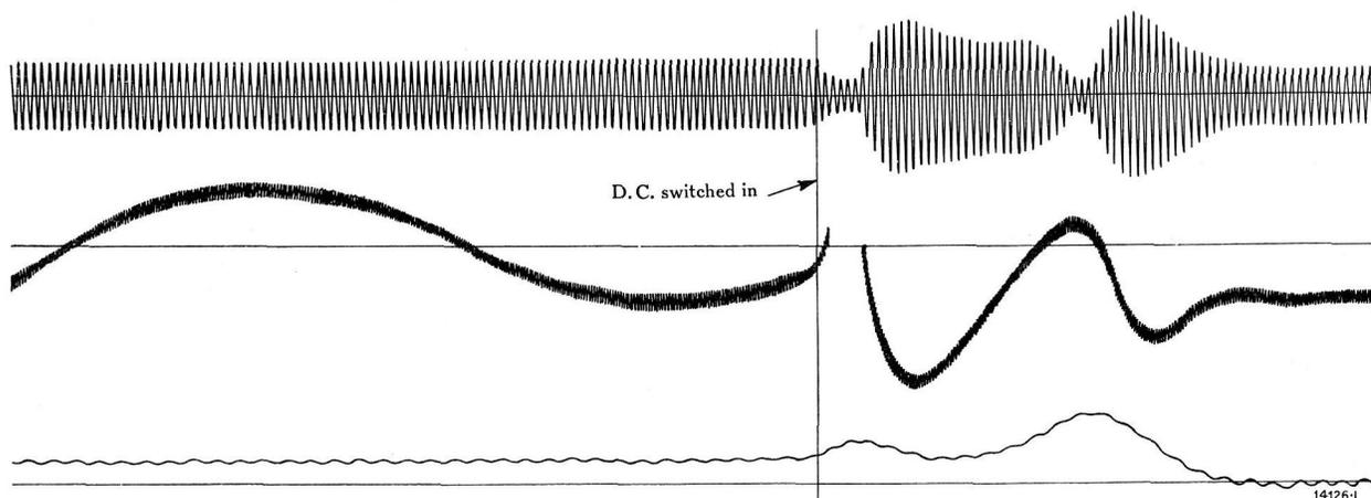
Fig. 11b. — Oscillogram showing the stator and rotor currents and slip during synchronization of a 1000-kW motor-generator set. Switching in takes place in the most unfavourable position.
