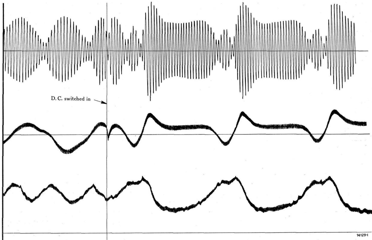
Fig. 13. — Oscillogram showing hunting when the motor is not pulled into step.
