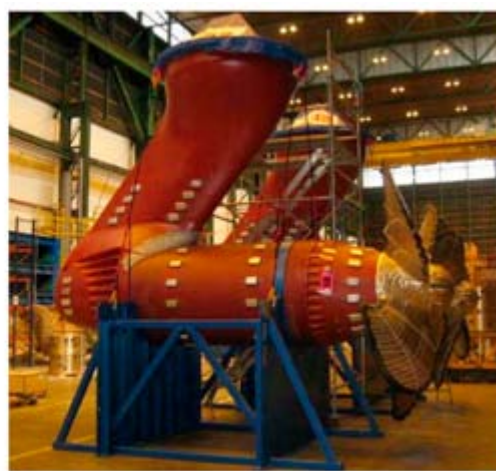
Figure 5-5 Operating area and Azipod propulsors ready for original shipment from Helsinki
