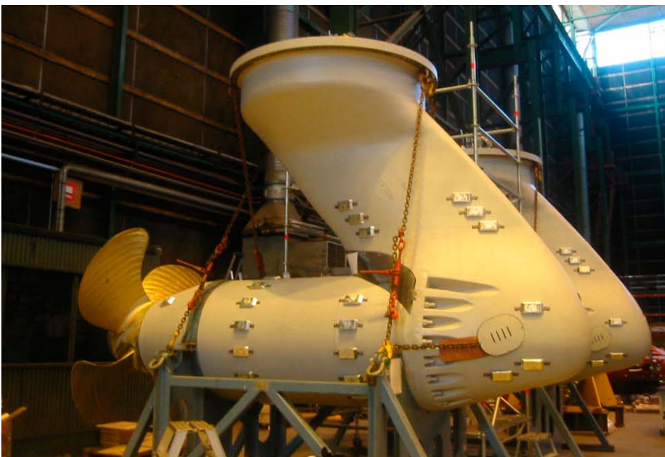
Figure 5-7 CO steering propulsors for “Ice” ready for dispatch to the Lürssen shipyard
