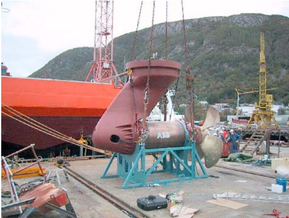
Figure 5-3 Azipod CO1400 propulsor ready for installation at Søviknes Verft.
