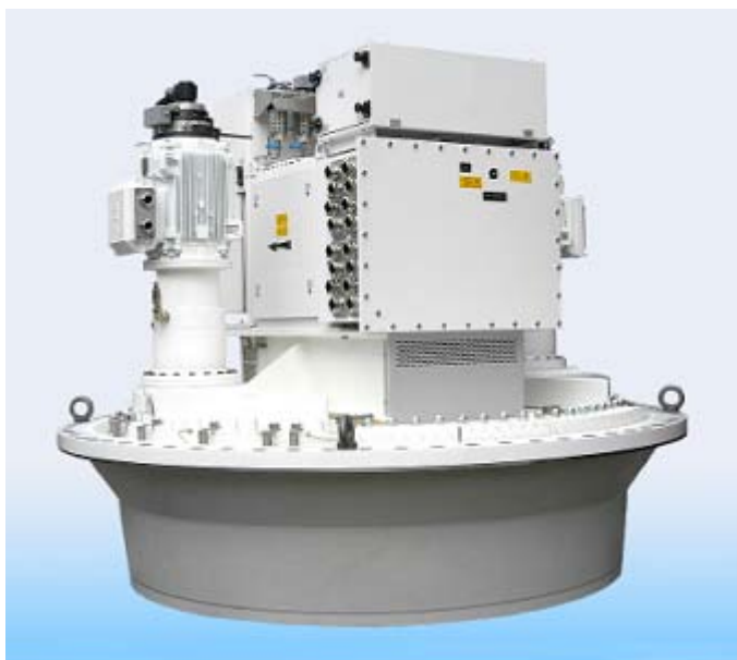
Figure 2-2 Steering Module ready for packing and for delivery to the shipyard
