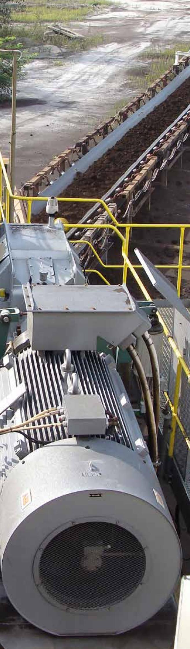
— 01 Typical conveyor drive with gearbox.
