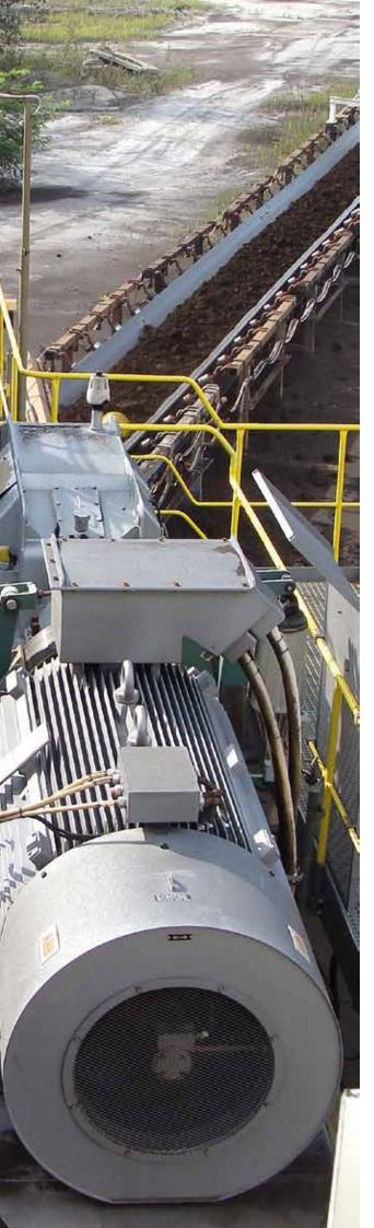
01 Typical conveyor drive with gearbox.
