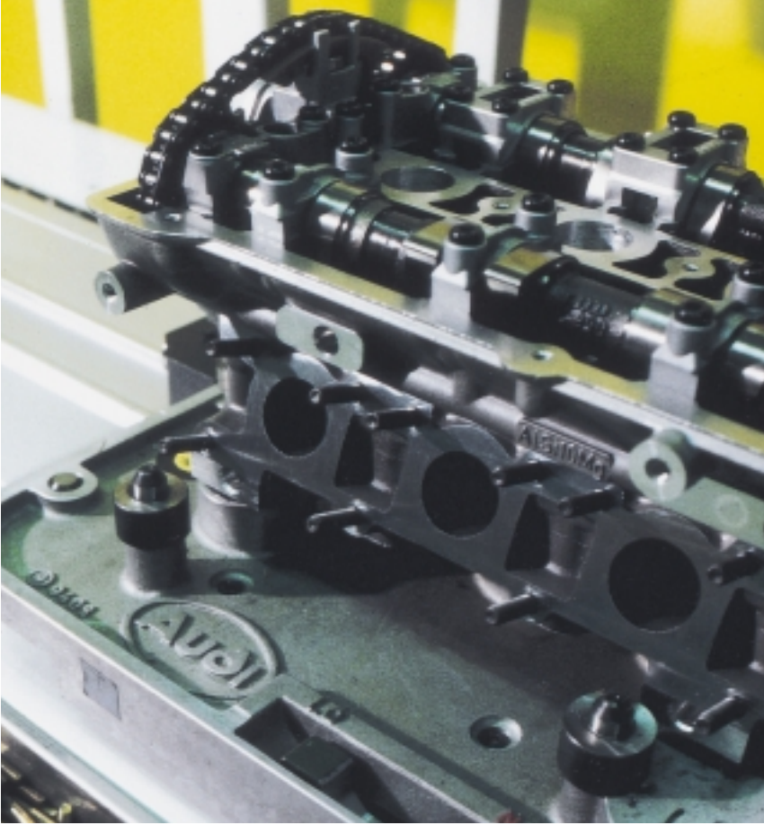
Multivalve cylinder head for an Audi car engine on the robotized assembly line at Győr, Hungary
