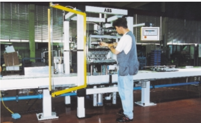
All the stations are easily accessible for maintenance and service work. The transparent enclosure, made of high-strength Macrolon, gives operators an uninterrupted view of all the key parts of the installation and the assembly process.
