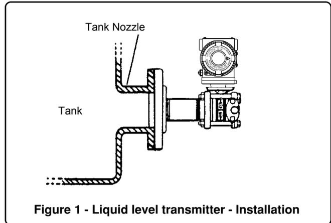
Figure 1 - Liquid level transmitter - Installation
