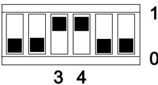
Switch 4 up in "1" position allows the replace of the secondary electronics. It must be moved in this position, when electronics replace is being performed, before power up the transmitter.
