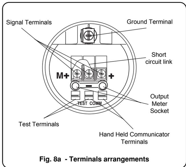
**WARNING :** DO NOT ATTEMPT TO CONNECT AN AMPEROMETER BETWEEN A "TEST" TERMINAL AND A "COMM" TERMINAL. THE RESULT TO THE POWER SUPPLY IS A SHORT WHICH WILL BLOW FUSES AND POSSIBLY DAMAGE YOUR EQUIPMENT, ALSO CAUSING TO INTERRUPT FUNCTION OF OTHER DEVICES POWERED FROM SAME SUPPLY.
