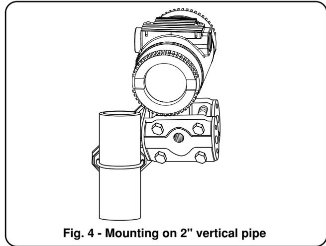
Fig. 4 - Mounting on 2" vertical pipe
