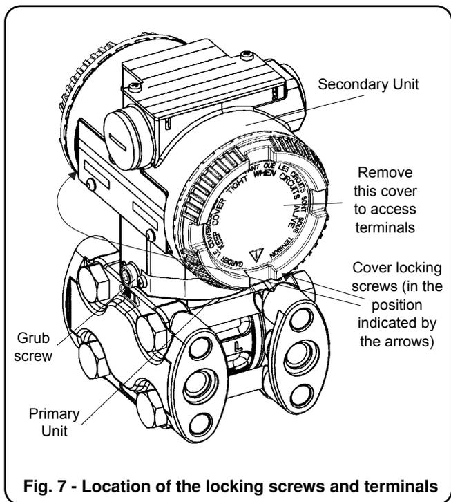
The power to the transmitter is supplied over the signal wiring and no additional wiring is required. The signal wiring does not need to be shielded but the use of a twisted pair is highly recommended. The cable shield should be grounded in one side only, to avoid dangerous earth paths.
