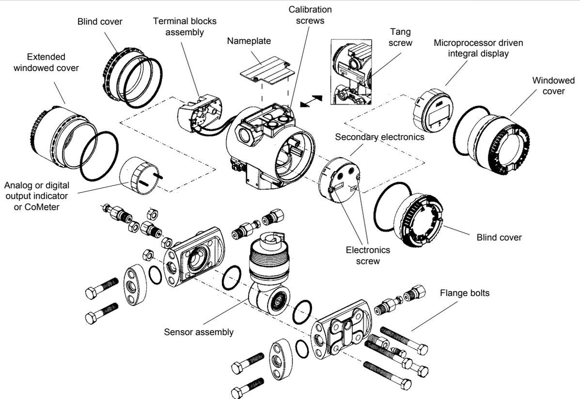
Fig. 13b - Transmitter Sectional View for model 264BS
