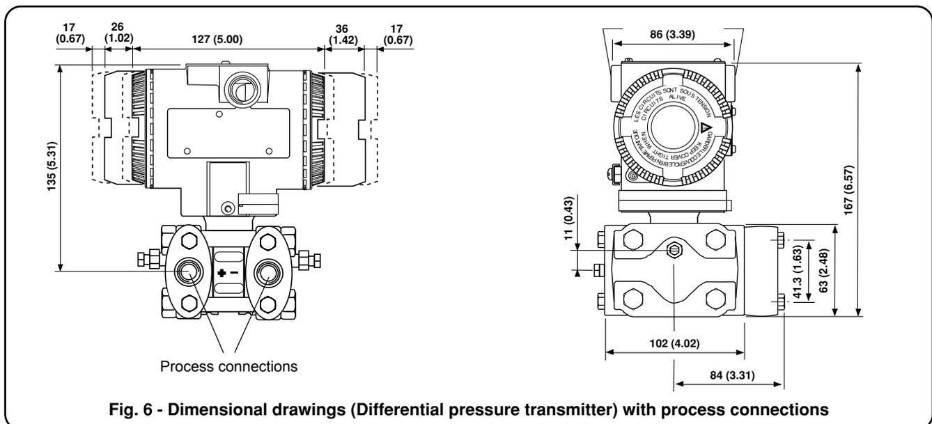
Fig. 6 - Dimensional drawings (Differential pressure transmitter) with process connections
