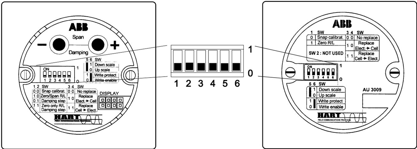
Switch 1 and 2 are used for Snap Calibration, Zero and Span Raise/Lower and also for Damping step.
