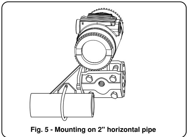
Fig. 5 - Mounting on 2" horizontal pipe
