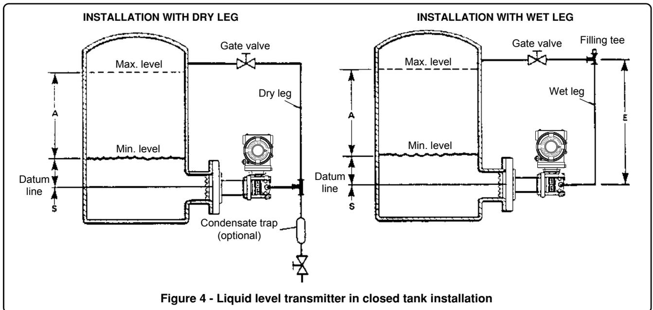
Figure 4 - Liquid level transmitter in closed tank installation
