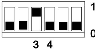
Switch 3 up in "1" position is required before power up the transmitter, when a replace is being performed. Switch 4 down in "0" position allows the replace of the transducer.
