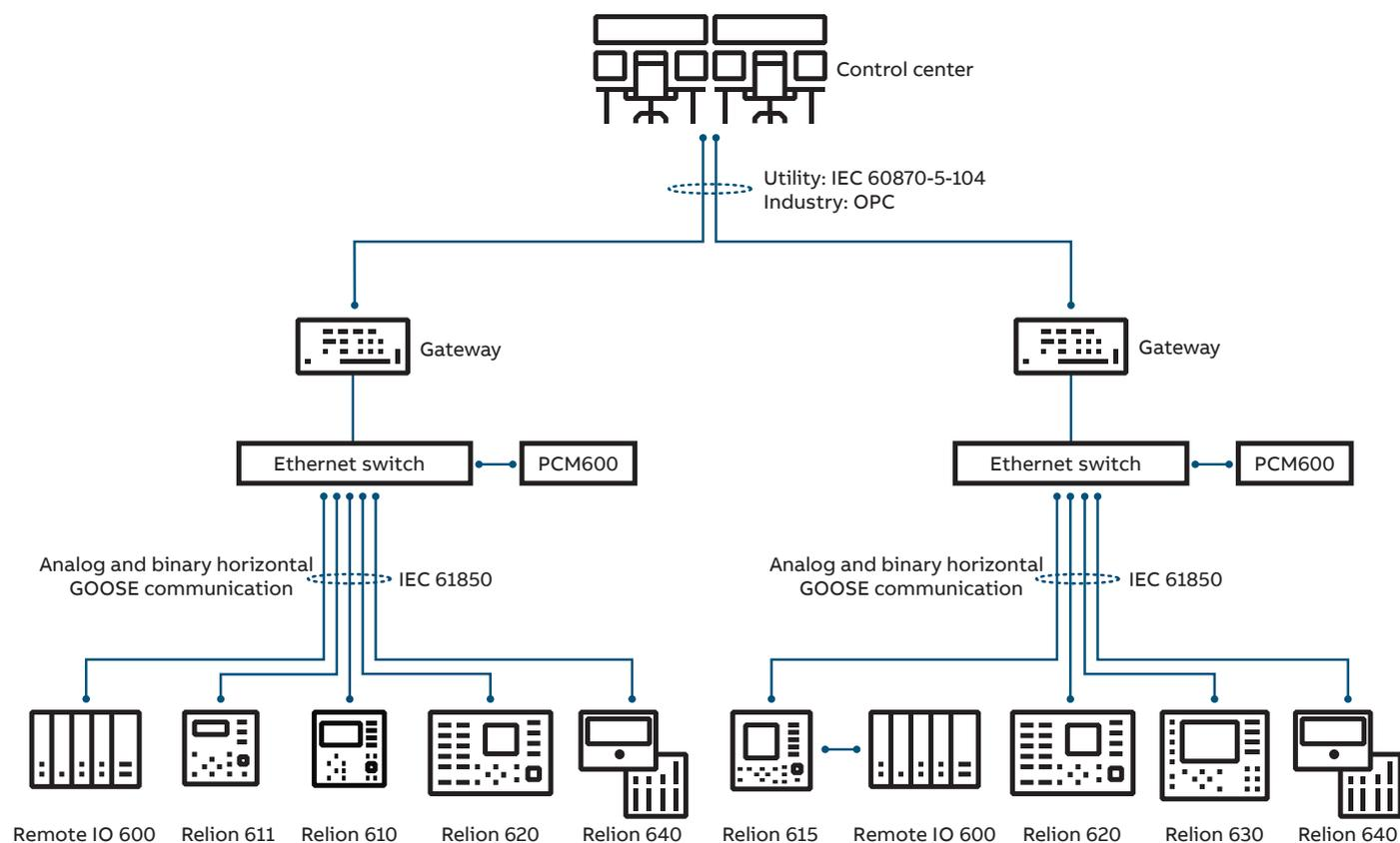
Figure 6. Communication example using Relion relays
