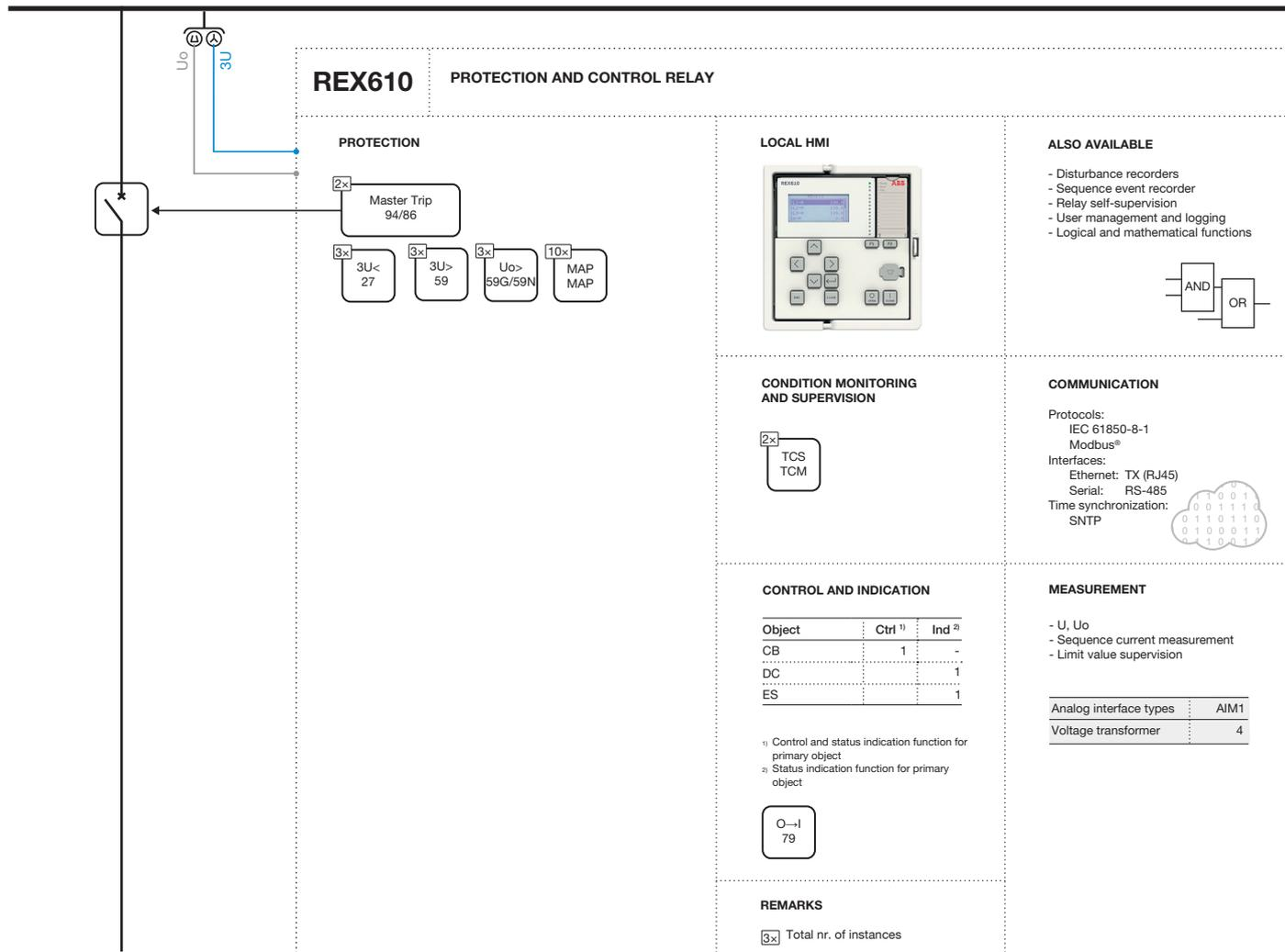
Figure 4. REX610 with VT module installed
