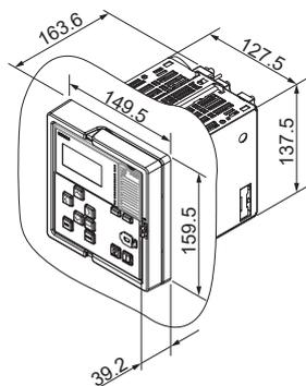
Figure 8. Flush mounting
