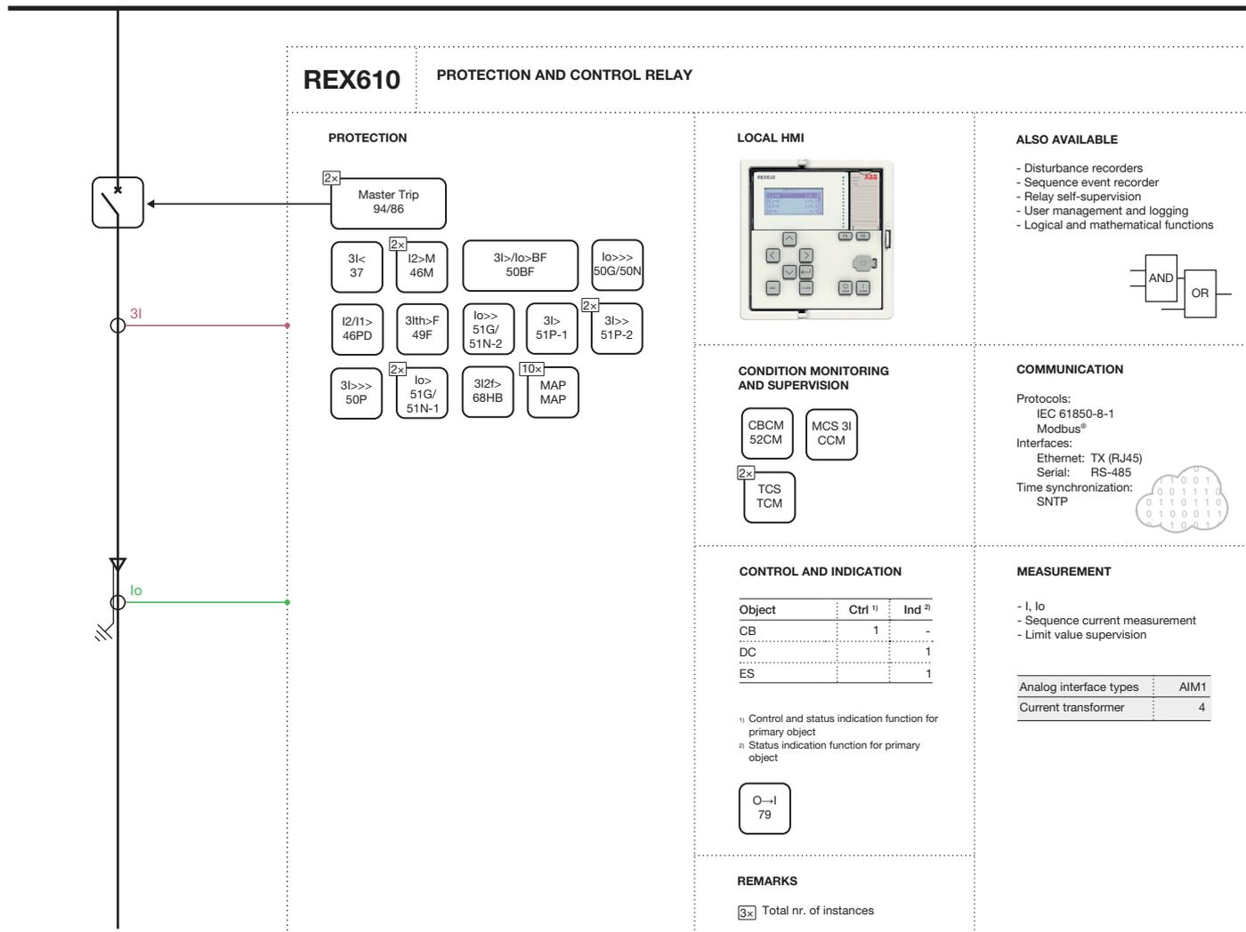
Figure 2. REX610 with CT module installed
