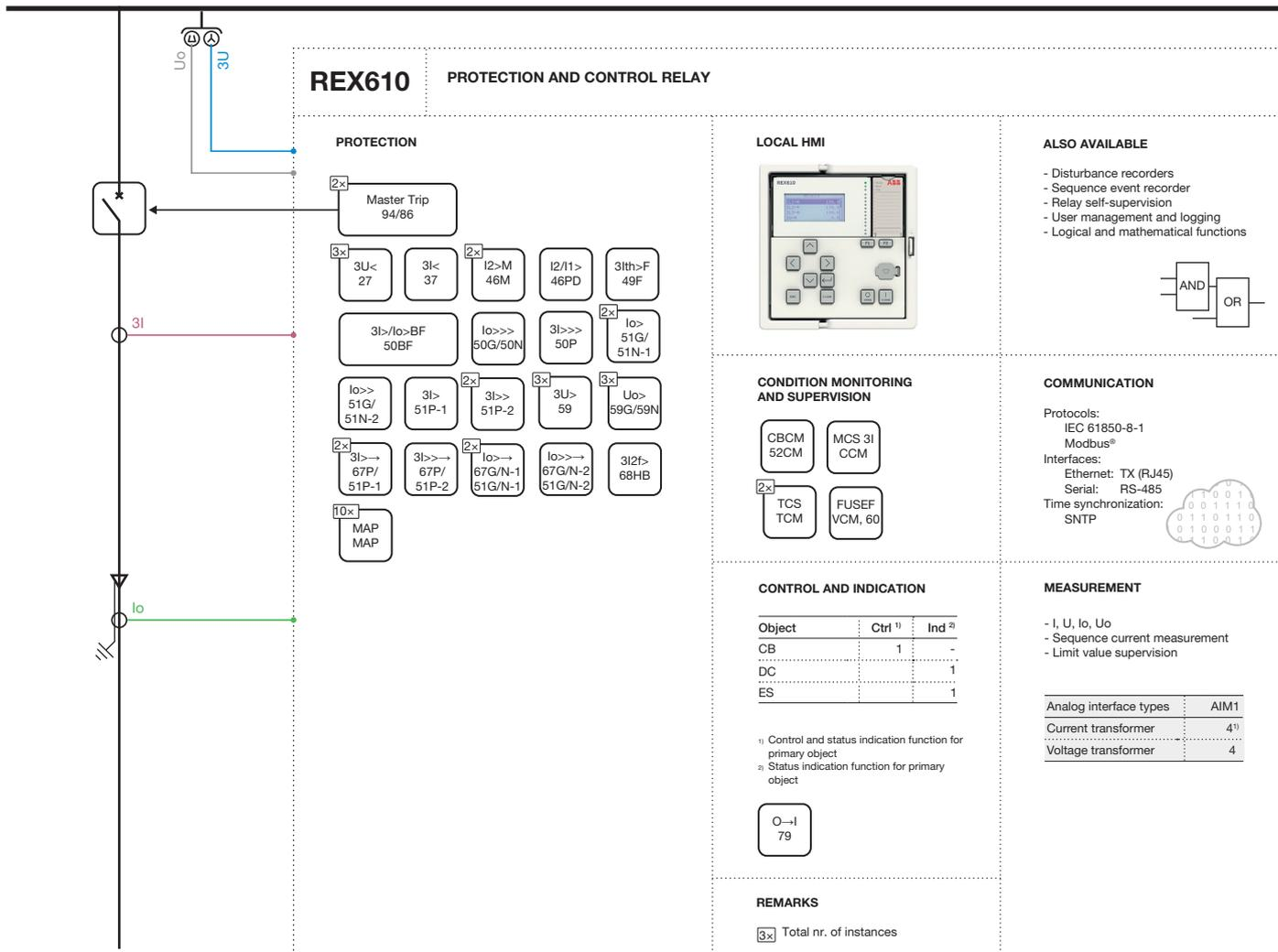
Figure 3. REX610 with CT and VT modules installed
