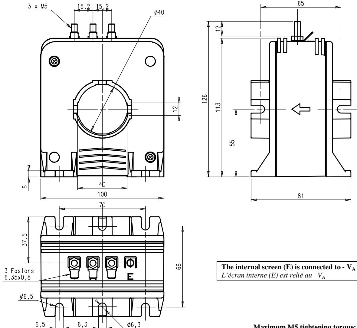
Maximum M5 tightening torque: 2 N.m
