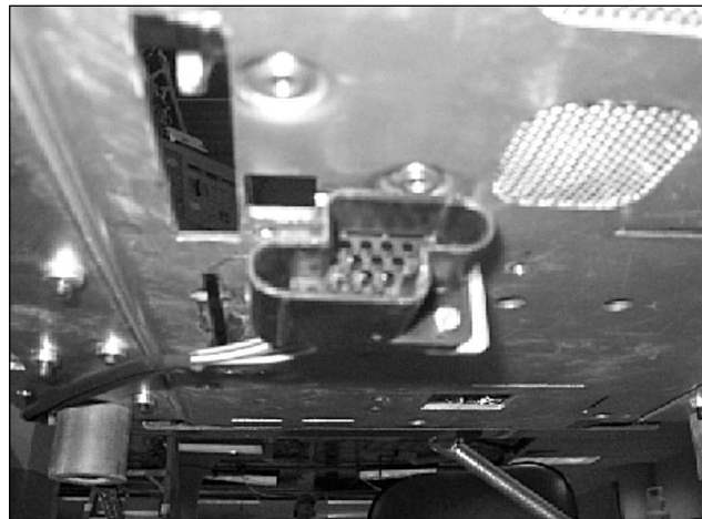
Figure 30. AKD-6 AKR30H\50H—19-Pin Disconnect Assembly (Compartment Side)
