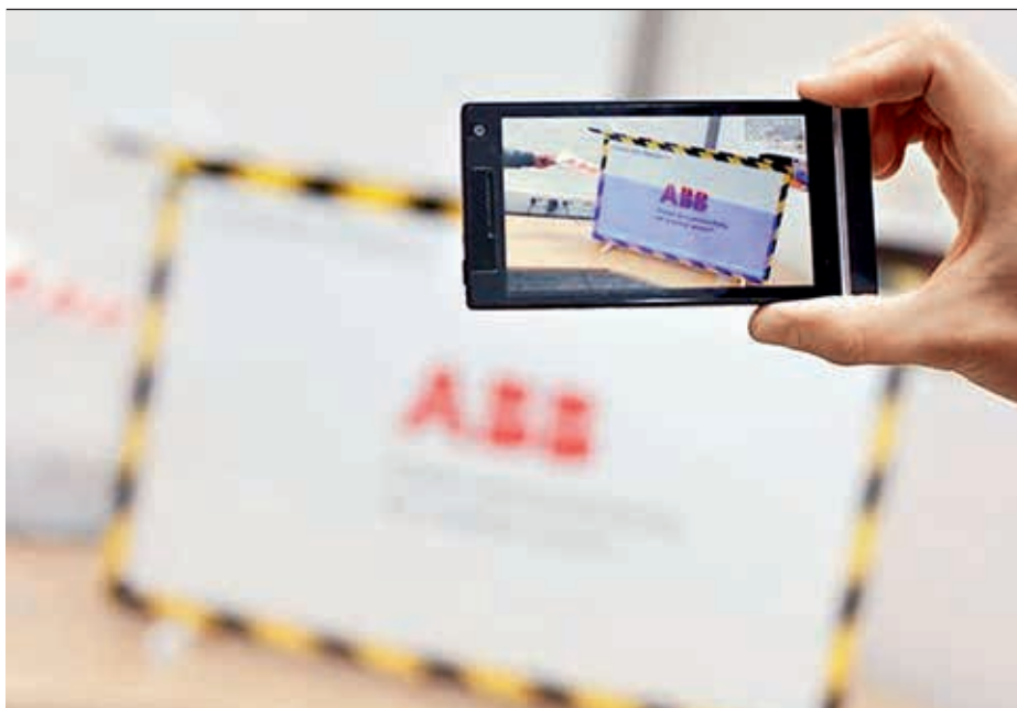
2 The prototype for showing tank values in a camera view of a mobile device
