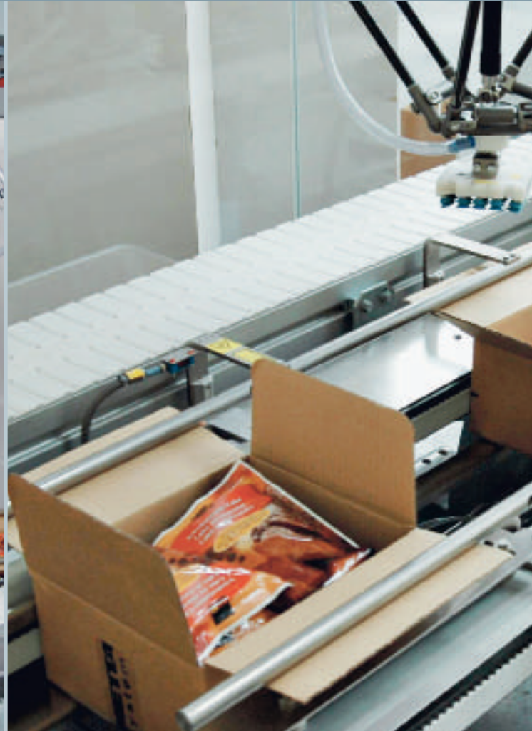
The Skinetta end-of-line packaging machine packages up to 88 bags per minute.
