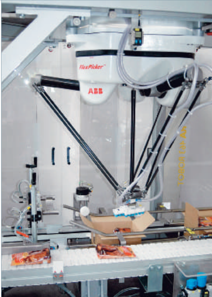
The RobTeq Speed-Picker packages bags weighing up to 1,000 grams. The suction technology of the ABB Flex-Picker was optimized in order to achieve this.
