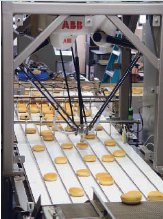
Hamburger buns bound for McDonald's get inspected by an IRB 340 robot at Northeast Foods.
