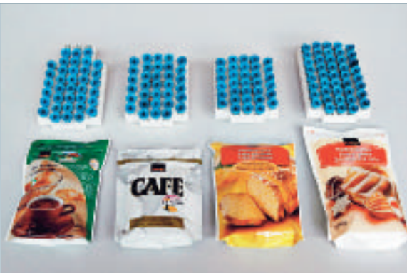
Suitable suction heads have been developed for the different bags which can be changed in seconds using a new type of clip fastening.
