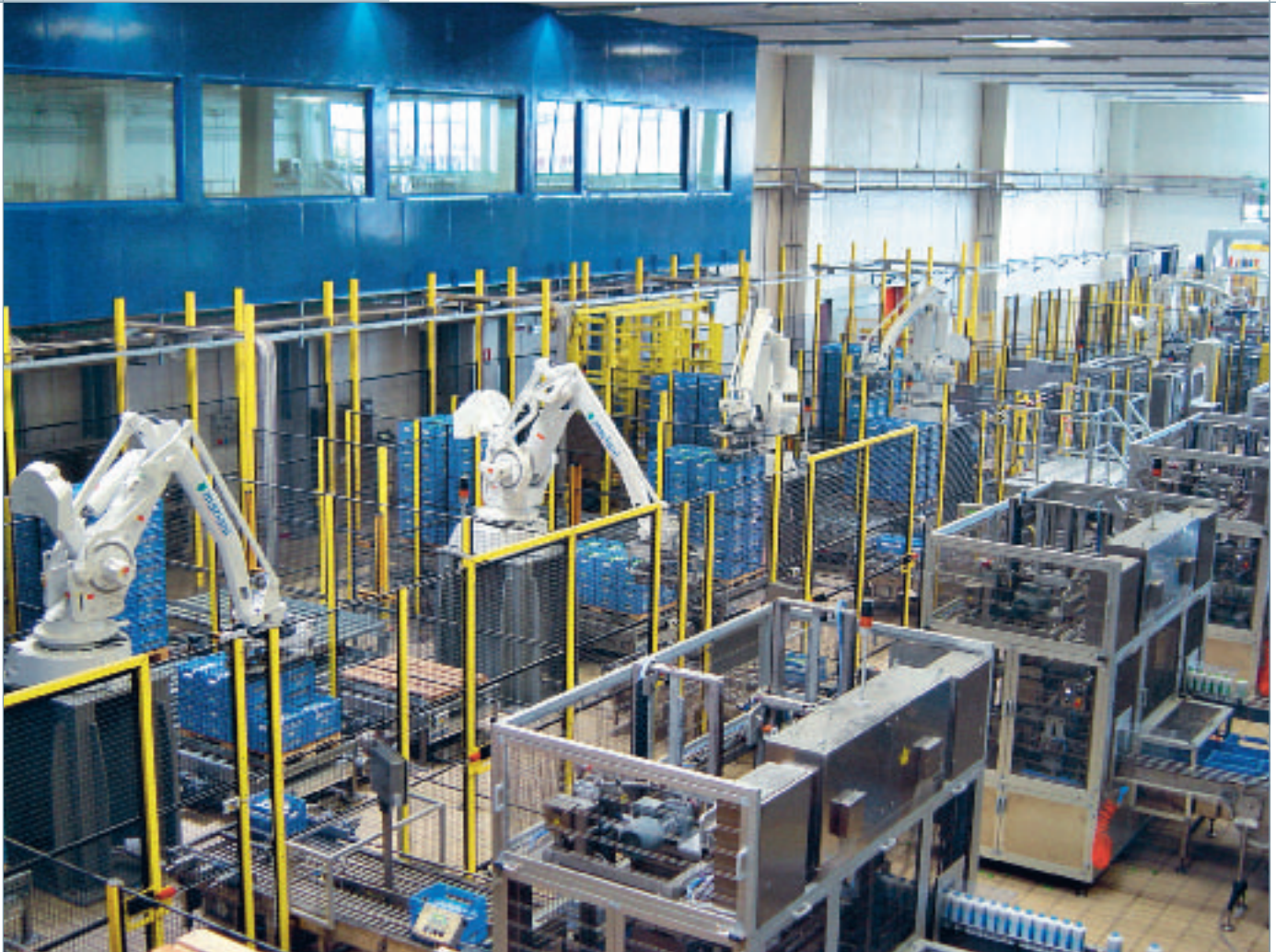
Four IRB 640 robots handle the palletizing of crates of dairy products received from the four packaging lines.
