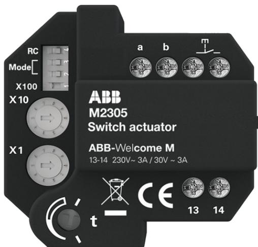
The switch actuator can be used to control equipment such as doorbells, garage doors, lights, etc. It can also extend the doorbell function and serve as a time relay. Up to 199 of these can be implemented in one system.
