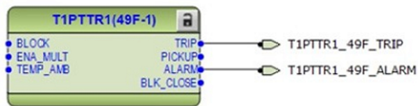
Figure 42: Thermal overload protection
