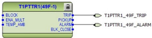
Figure 85: Thermal overload protection
