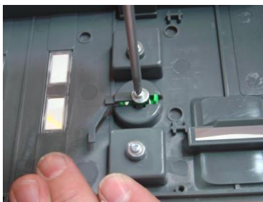
Fig 11. Push button assembly
