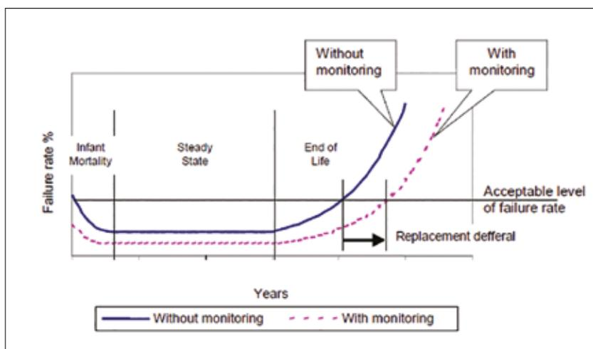
Figure 1. Bathtub curve, with and without monitoring
