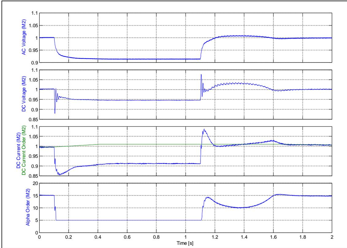
**Figure 2** – AC voltage drop at the LCC station, resulting in mode shift.
