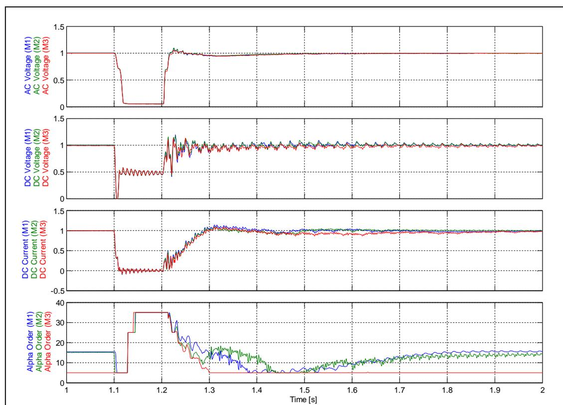
**Figure 3** – Three-phase to ground AC fault at the LCC station.
