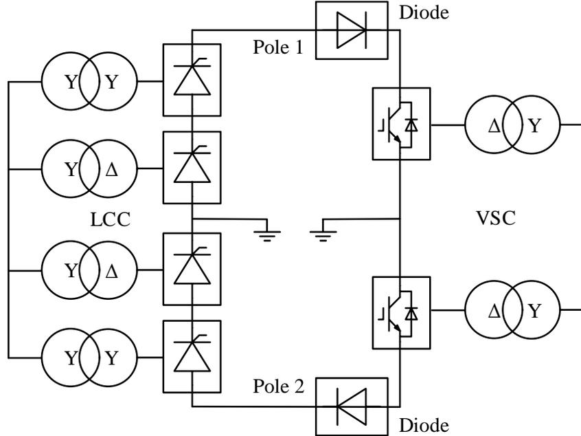
**Figure 1** – Overview of the tested hybrid HVDC system, including Diode
