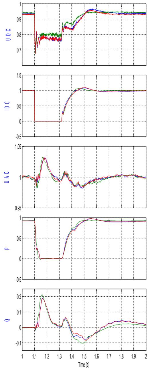
**Figure 5b** – DC fault, VSC response
