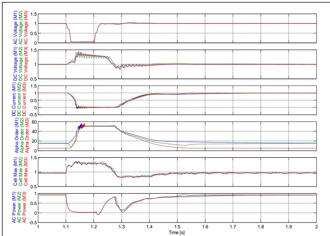
**Figure 4** – Three-phase to ground AC fault at the VSC station.
