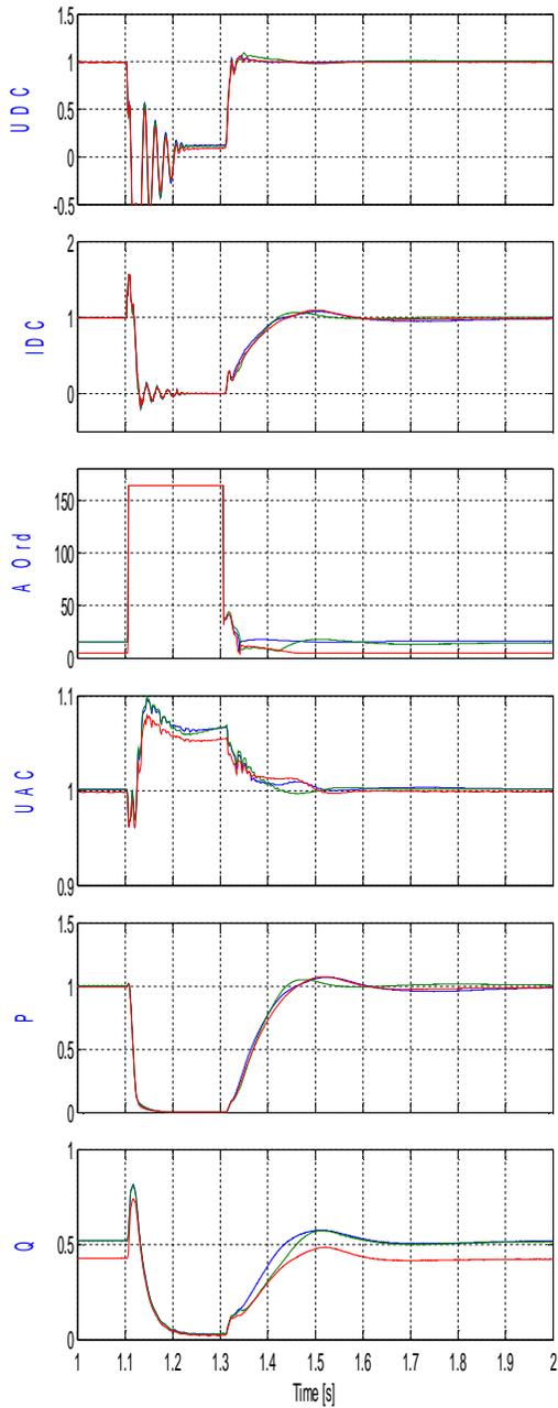
**Figure 5a** – DC fault, LCC response
