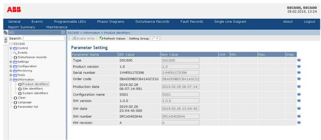
Fig. 2 Current firmware revision of the SSC600 product
