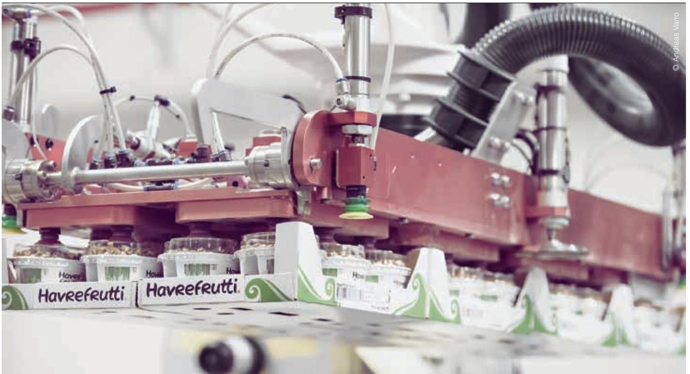
When a pallet is full, the robot changes function and uses the gripper to lift the new pallet into place. The robot can fill one pallet in 10 minutes, corresponding to a total of 8,500 products an hour.
