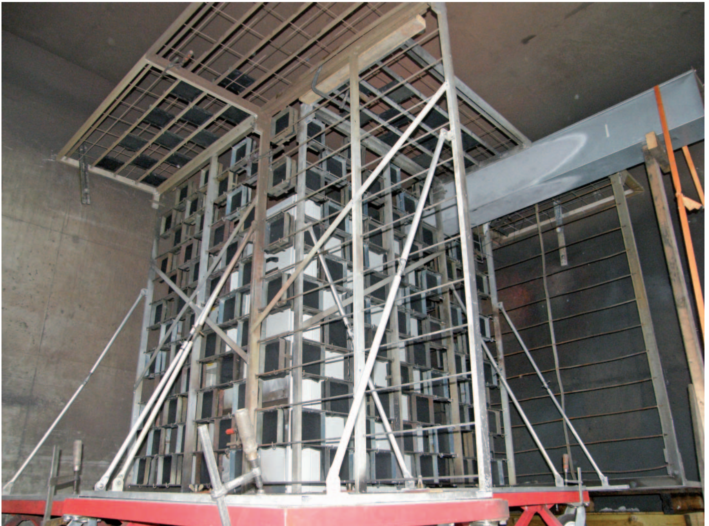
Setup for an internal arc withstand test
