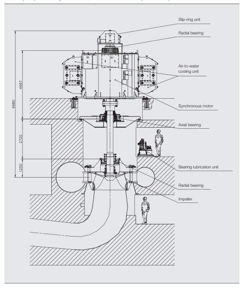
Pumping is typically performed at a constant speed, and the combination of high power and low speed makes a synchronous motor the most economical choice in lift irrigation projects.
