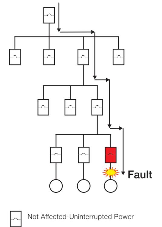
Figure 2. Systems providing breaker coordination
