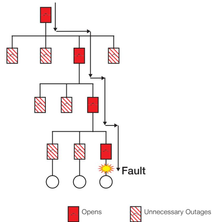
Figure 1. Systems lacking breaker coordination
