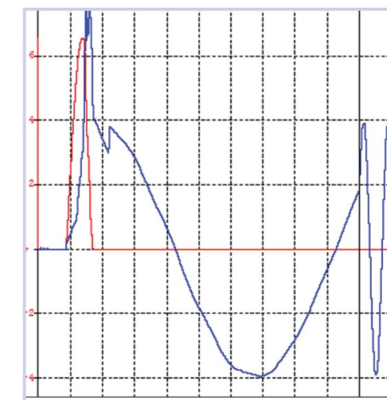
In this example of selective coordination the graph shows the response to short circuit of 26.8 kA (almost 3X the rated capacity) of an ABB S200 current-limiting breaker (red line). Compared to a zero-crossing breaker, which could require as long as 8.3 milliseconds, the current limiting breaker tripped in 1.7 milliseconds, one-quarter of an AC cycle. The upstream breaker (blue line) never saw enough energy to trip, remaining closed and operational.
